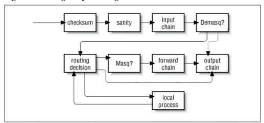
Figure 9.8: Datagram processing chain in IP chains
