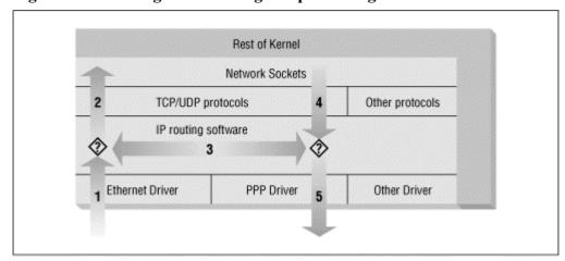
Figure 9.2: The stages of IP datagram processing
