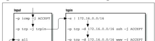
Figure 9.7: The rules flow for a received TCP datagram for telnet
