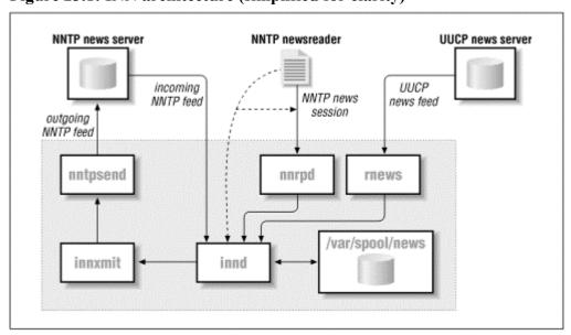
Figure 23.1: INN architecture (simplified for clarity)
