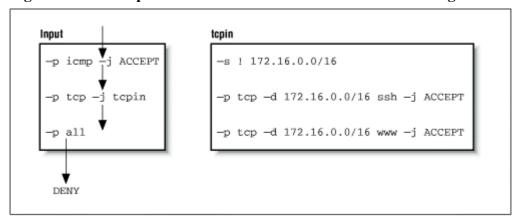
The datagram is received by the input chain and falls through the first two rules because they match ICMP and TCP protocols, respectively. It matches the third rule in the input chain, but it doesn't specify a target, so its datagram and byte counters are updated, but no other action takes place. The datagram reaches the end of the input chain, meets with the default input chain policy, and is denied.
