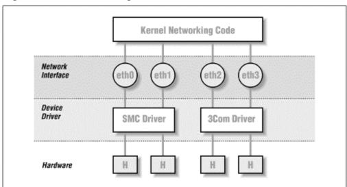
Figure 3.1: The relationship between drivers, interfaces, and hardware
