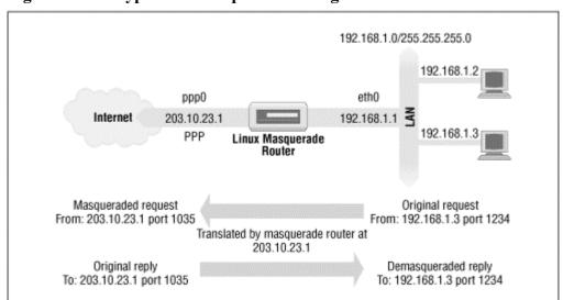
Figure 11.1: A typical IP masquerade configuration
