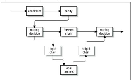
Figure 9.9: Datagram processing chain in netfilter
