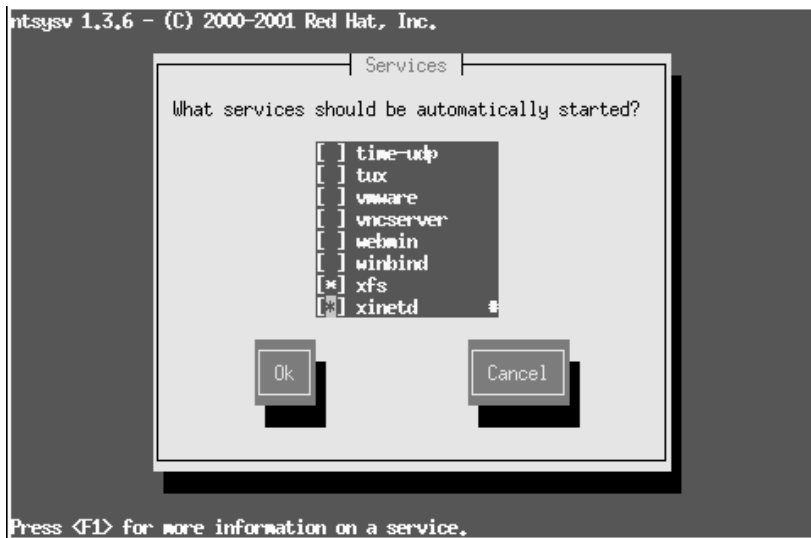
Figure 8-5 Use the ntsysv command to determine which services start when the system boots.
