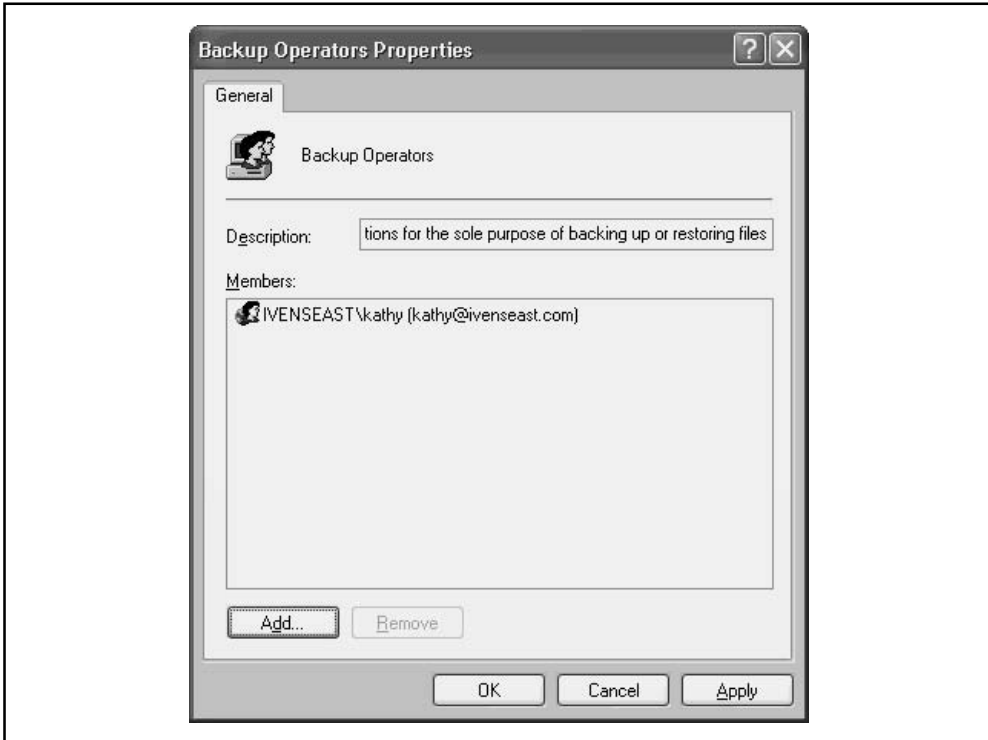
Figure 20-2. The membership list displays the location (local or domain) and FQDN of each member.
