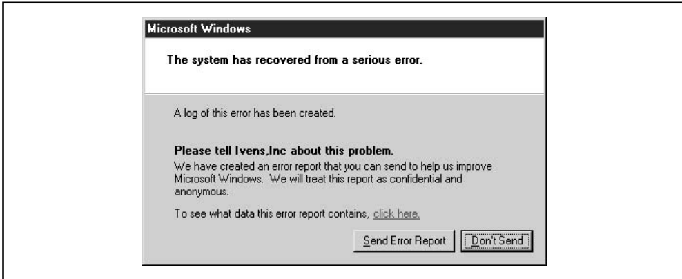
Figure 26-12. This message asks the user to notify the company instead of Microsoft as a result of the group policy that substitutes another term for “Microsoft” in error dialogs.
