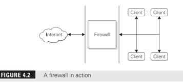
that match the rules. Rules include checking the port number (TCP or UDP), for example, blocking all ports except port 80 (HTTP for Internet access) and redirecting certain ports, for example, redirecting any port 25 traffic (SMTP for e-mail transfer) to a specific host within the network (your mail server).
