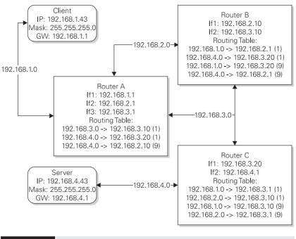
FIGURE 5.1 A sample routed network showing the routing tables
