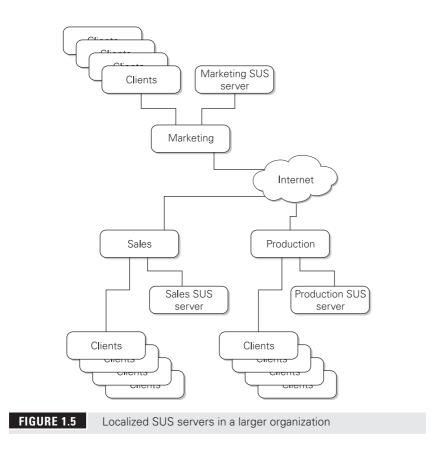
By approving updates on the central server, the two servers downstream receive all the updates. However, updates to the web servers and updates to the clients can be independently controlled by approving individual updates on each of the downstream servers. This allows you, for example, to install patches for known exploits on the web servers immediately, as these are public facing, while waiting until further tests have been completed before approving the same update for your clients.
