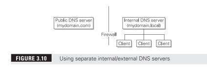
In this situation in Figure 3.10, there is no communication between the internal and external servers. However, the same principles of an internal-only DNS server apply: you must configure your internal server to host the top-level and root domains.
