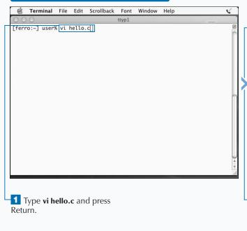
Terminal File Edit Scrollback Font Window Help #include <stdio.h> main () { printf("Hello, World\n"); \*Append 2 Press I and type #include 3 Type main () { and press <stdio.h>, then press Return Return, then press the Tab key and type printf("Hello, twice. World\n"); and press Return The include command adds the standard IO header 4 Type } and press Esc, then file to your program. type:wq.
