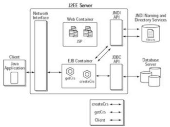
Figure 16–5: An example application architecture using CachedRowSet objects
