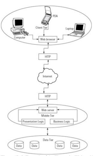
Figure 17–3: Example of the Three–tier Web architecture
