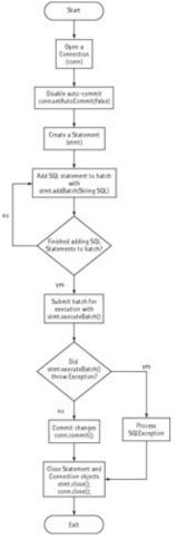
Figure 5–4: This flow chart shows JDBC batch processing.
