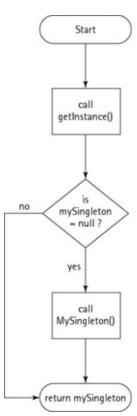
Figure 10–2: Flowchart of the Singleton pattern
