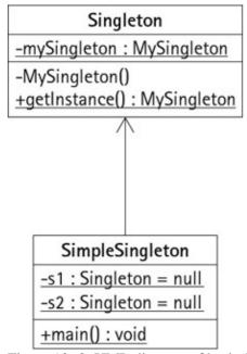
Figure 10–3: UML diagram of basic Singleton example
