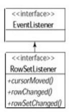
Figure 16-4: UML class diagram of the RowSetListener interface
