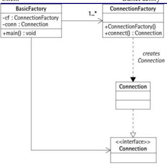
Figure 11-2: UML class diagram of BasicFactory method example
