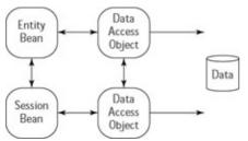
Figure 19-9: Using data access objects
