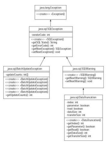
Figure C-1: UML class diagram of JDBC Exception classes
