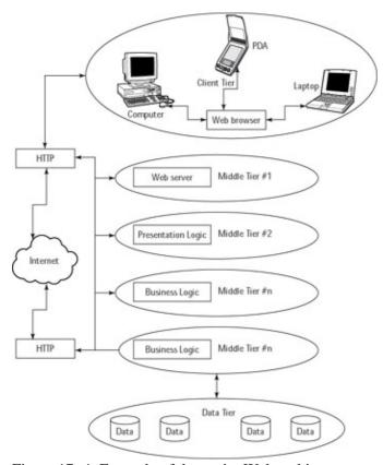
Figure 17–4: Example of the n-tier Web architecture
