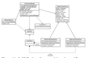
Figure 11–3: UML class diagram of the enhanced Factory Method example
