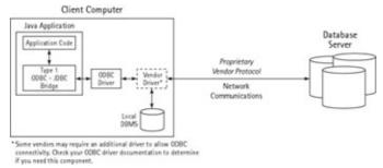
Figure 4–3: JDBC Type 1 driver: JDBC–ODBC bridge
