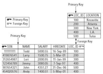
Figure 2–4: Example of a foreign key
