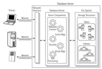
Figure 2-1: Conceptual view of an RDBMS
