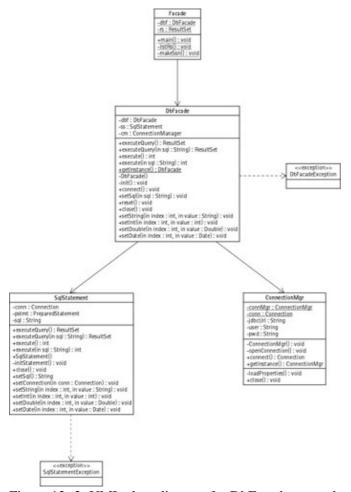
Figure 12–2: UML class diagram for DbFacade example
