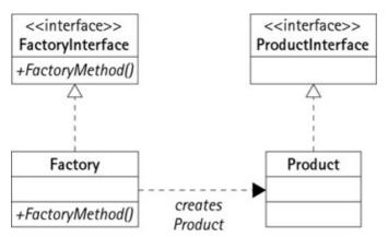
Figure 11–1: UML class diagram for the Factory Method pattern
