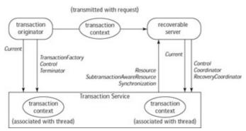
Figure 15–3: Major components and interfaces of the Transaction Service
