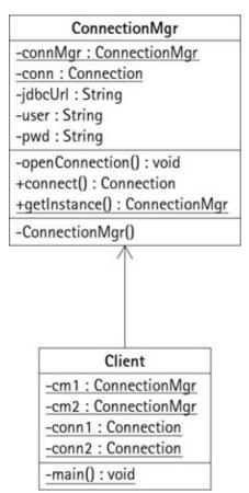
Figure 10-4: UML class diagram for Connection Manager Singleton
