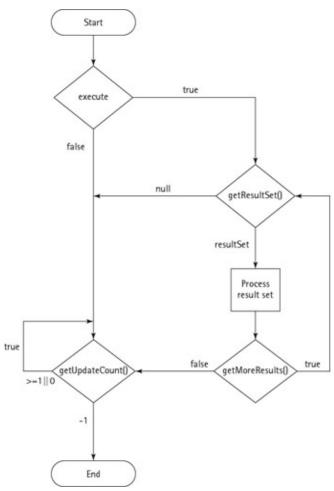
Figure 5–3: This flow chart shows how to process the results from the execute() method.
