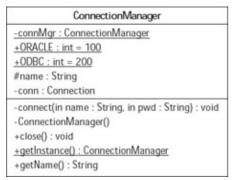
Figure D-2: ConnectionManager UML classdiagram
