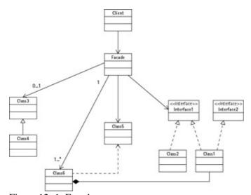
Figure 12-1: Façade pattern structure
