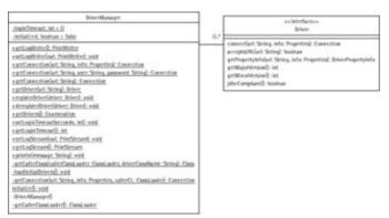
Figure 4–7: UML class diagram of Driver and DriverManager
