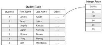
Figure 7–2: Example of SQL ARRAY data type
