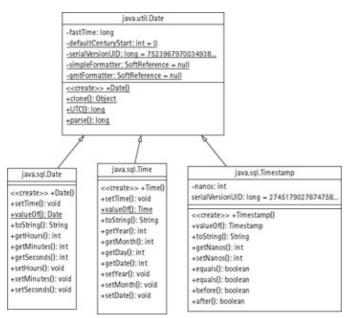
Figure 7–1: UML class diagram for JDBC Date and Time classes
