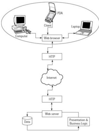
Figure 17–1: Example of the two–tier Web architecture
