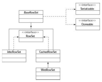
Figure 16–1: UML class diagram of the RowSet reference implementation
