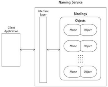
Figure 13-1: Conceptual view of a naming service
