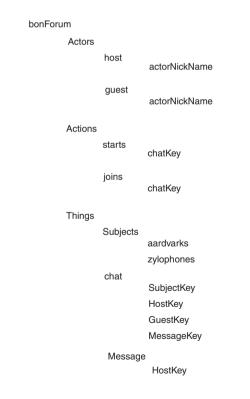
Figure 5.4 Designing bonForum XML using a tree diagram.
