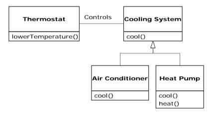
Of course, once you see this design it becomes clear that the base class "cooling system" is not general enough, and should be renamed to "temperature control system" so that it can also include heating—at which point the substitution principle will work. However, the diagram above is an example of what can happen with design in the real world. Feedback
