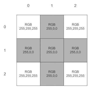
Figure 6-8. A pixel-by-pixel image
