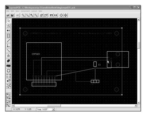
Figure 4-4. Schematic of CMPS03 board with ExpressPCB software
