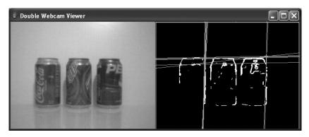
Figure 6-24. The Hough transform of the three cans
