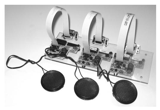
Figure 4-16. Three Polaroid 6500 Ranging Modules with Transducers
