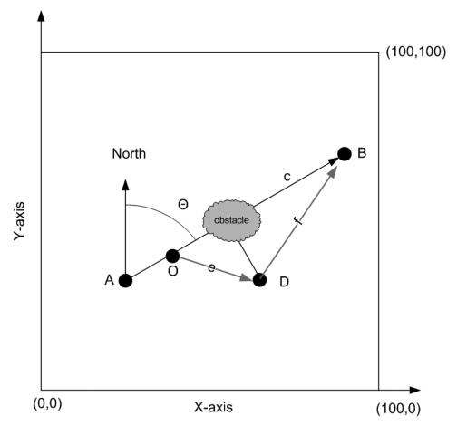
Figure 7-10. Obstacle detection and path planning
