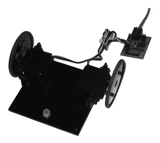
Figure 3-5. The differential drive of a CubeBot
