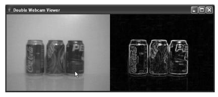
Figure 6-23. The Sobel Gradient filter
