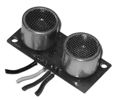
Figure 4-15. The Devantech SRF04 Sonar Module
