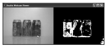
Figure 6-13. The red threshold
