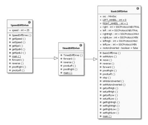
Figure 7-7. The SpeedDiffDrive class diagram from Chapter 2
