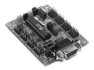
Figure 3-9. The Lynxmotion SSC-32 Servo Controller
