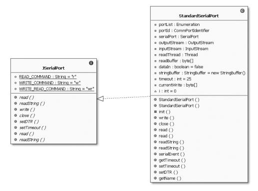
Figure 2-3. The class diagram for JSerialPort and StandardSerialPort
