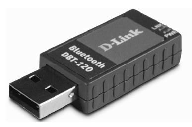
Figure 2-10. DLink DBT-120 USB Wireless Bluetooth Adapter
