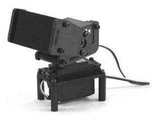
Figure 3-7. The Lynxmotion Pan and Tilt Kit
