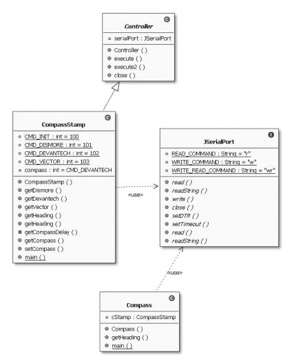
Figure 4-10. A class diagram relationship to the Chapter 2 classes
