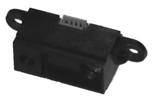
Figure 4-14. The Sharp Infrared GP2D02
