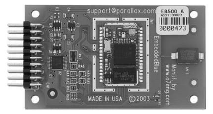
Figure 2-9. The Parallax EB500 Bluetooth Transceiver Module
