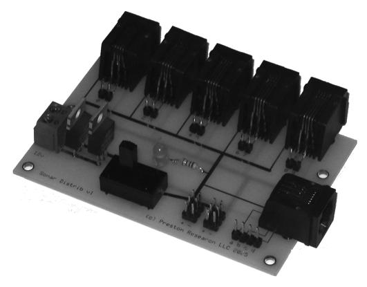
Figure 4-6. The Preston Research Sonar Distribution Board
