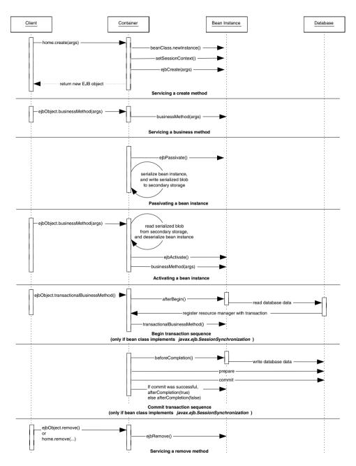
**Figure E.6** Sequence diagram for stateful session beans. For simplicity, the Container object represents all container subsystems, including EJB objects, home objects, transaction services, and so on.
