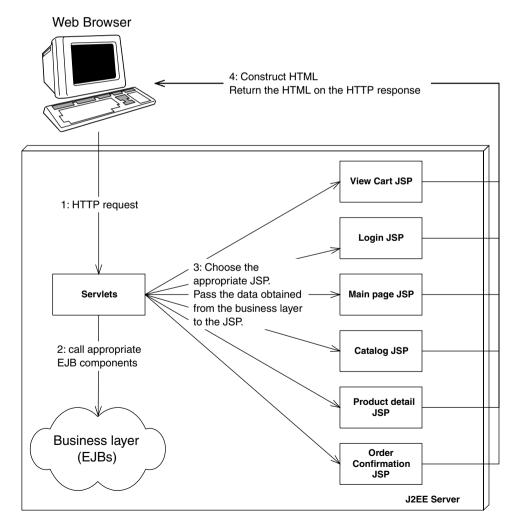
Figure 17.11 The EJB-JSP-Servlet Model-View-Controller Paradigm.
