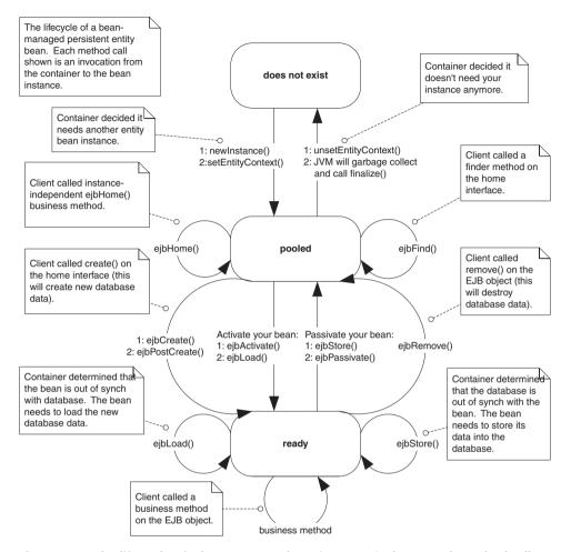
**Figure E.8** The life cycle of a bean managed persistent entity bean. Each method call shown is an invocation from the container to the bean instance.
