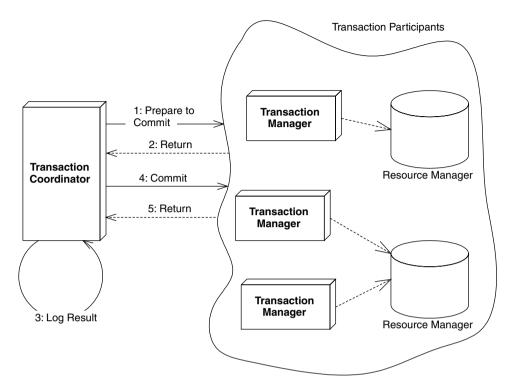
Figure 10.9 A distributed flat transaction using a two-phase commit protocol.
