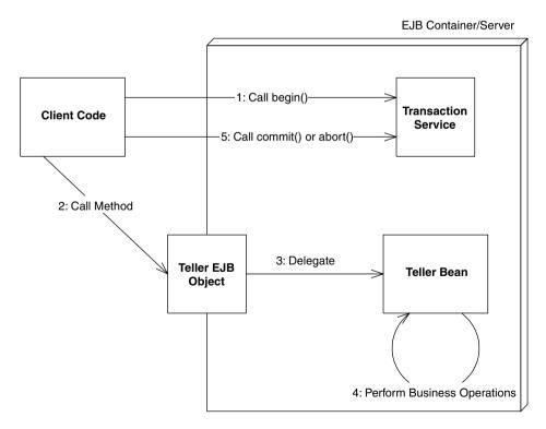
Figure 10.7 Beans with client-initiated transactions.
