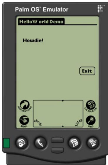
Figure 15.1 The VAME HelloWorld application is depicted here running on IBM's J9 virtual machine in a Palm OS device. VAME allows developers to make native OS calls at the expense of portability.
