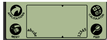
Figure 9.14 The Graffiti Area is located at the bottom of the Palm OS screen. The left side of the Graffiti Area is used for entering characters. The right side is for entering numbers. In either case, one must be familiar with the Graffiti shorthand in order to enter information.
