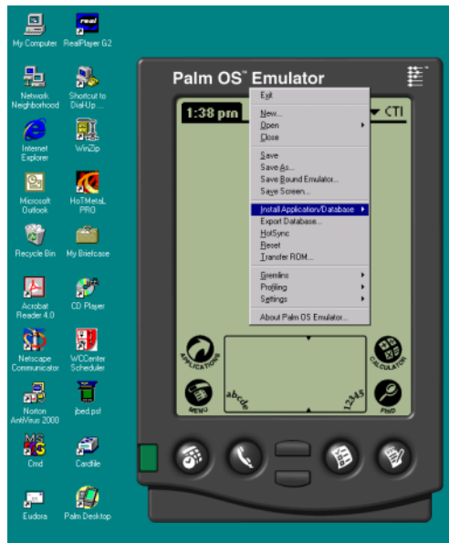
Figure 8.20 Right-click anywhere on the emulator application to get the emulator's menu. This menu provides the options to load applications and databases among other options.
