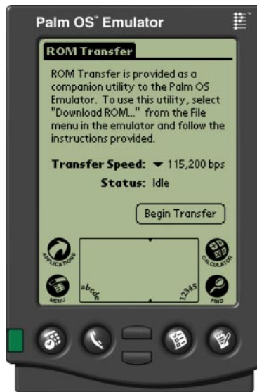
Figure 8.19 When the desktop has been set up appropriately to receive the ROM image from the device via the cradle, push the Begin Transfer button, as seen in this picture, to send the ROM image of the device to the emulator on the computer.
