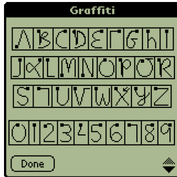
Figure 9.15 Graffiti help like this is displayed when the stylus is dragged from bottom to top on the device screen. The help shows how to enter the various characters and numbers by providing an indication of where the stylus must be started and how to drag it across the Graffiti Area to get the desired input.
