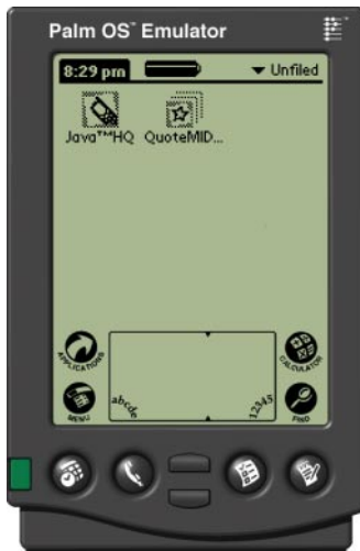
Figure 5.34 The MIDP Investment Quote MIDlet suite is represented by the QuoteMID... icon displayed on the Palm after completing conversion and deploying. The JavaHQ icon displayed in this screen is the virtual machine PRC on the Palm OS device.
