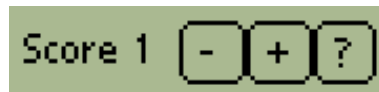
Figure 9.16 A ValueSelector allows for integer value entry. In the figure displayed above, the ValueSelector has a label of Score and a current value of 1. The “-” and “+” buttons will increment and decrement the value respectively. The “?” button, when pushed, sets the value to a randomly assigned value.
