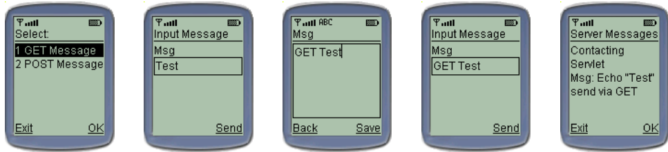
Figure 12.1 Running the EnterpriseClient application to perform a GET request. First the user selects “GET Message” from the main menu. Then the user enters a message to send and invokes the Send operation. The message is sent using an HTTP GET method and the response from the server is displayed.
