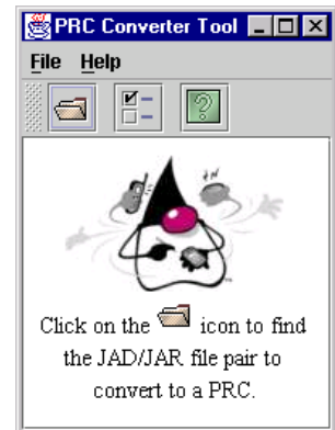
Figure 8.29 The MIDP for Palm OS PRC Converter tool allows MIDP JAD/JAR files to be converted to Palm OS PRC files. Running converter.bat starts Sun's MIDP for the Palm OS Converter Tool. Use the File menu to locate and open a MIDlet Suite JAD file for conversion.
