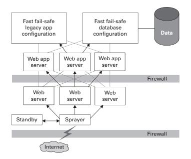
Figure 10.1 A good topology for performance has layers that do one thing and do it well. This one has a sprayer, with a hot standby, that takes incoming requests and routes them to one of three identical web servers. The web server can then request services to build dynamic content from any of the available web application servers behind the corporate firewall, which in turn can use database or transactional servers.
