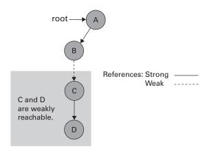
Figure 6.3 Weak references can be used to assist the garbage collector. An object is weakly reachable if it can be reached only through a weak reference. Weakly reachable objects are candidates for garbage collection.
