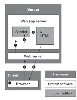
Figure 3.4 1 The user makes a request for a servlet. 2 The browser does an HTTP POST. **③** The web server passes the request through to the application server, possibly installed as a web server plug-in. **(4)** The application server invokes the servlet. **(5)** The servlet executes and prints out an HTML page that 6 is returned to the user.
