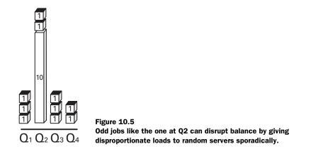
10 units, but because the second queue received additional work, the total length of time required to process all of the work was 12 units. Our throughput has suffered. In addition, our average waiting time has been extended to 7 units, because smaller jobs have to wait for larger ones to complete.
