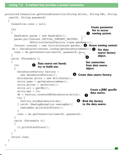
• Our data source will be a named resource, so we need to get a context. The parameters to the context constructor are stored in a hash table, which is then passed to the constructor. We'll use the context to find the data source that we create in steps 7 and 8.
