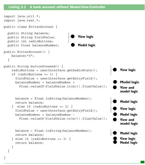
This application is the logic for a simple ATM program. It takes the amount in an entry field and debits or credits the account appropriately, based on the state of a radio button. Notice that no attempt has been made to break out the business logic (the account) and the user interface. In fact, the model and view are so tightly intertwined that, in many places, both the model and view are Bitter servlets
