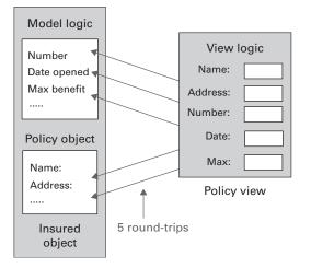
Figure 10.2 Round-tripping is considered the top EJB performance problem by many consultants. It occurs when significant iterations occur over major interfaces. In this case, we iterate through a list of fields, and set or get them independently across a client-server boundary.
