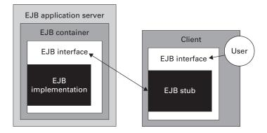
Figure 8.1 EJBs use client-side stubs to communicate with server-side objects. Users of the client-side EJBs use the remote interface, which in turn uses the proxy, which then uses the distributed interface and the local implementation. The server supports a container, which provides critical features to EJB components.
