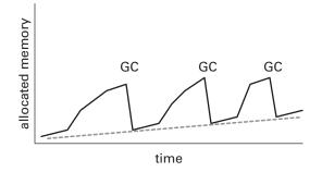
Figure 6.5 This is the classic resource chart of a memory leak. The solid black line shows actual memory use. The broken line projects reachable memory objects. The peaks and valleys are caused by garbage collection. The slowly rising valleys are characteristic of memory leaks.
