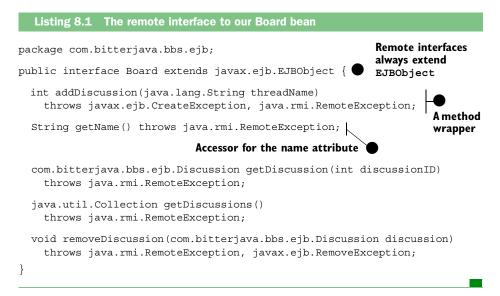
For a distributed persistent object, the interface is remarkably simple. We aren't forced to deal with the complexities—the container in our application server masks all of those complexities from us. Here we can see the power of the EJB architecture.
