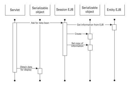
Figure 8.6 This sequence diagram is characteristic of the facade design pattern. The distributed interface appears just before the session EJB. Note that the communication is reduced to a single call. (Actually, one additional call at lower levels is required to initialize the communication with the stateless session bean.)
