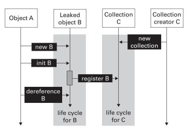
Figure 6.4 In the Leak Collection antipattern, an object with a short life cycle is registered in a collection with a long life cycle. Here we've shown a UML sequence diagram of such a memory leak. In this case, object B will be a memory leak, because the reference in collection C won't allow the garbage collector to free it.
