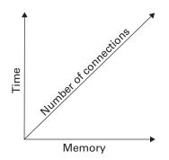
Figure 7.1 Consider the cost of connections. Each additional connection has fixed costs, in both units of time and system resources (such as memory). It isn't unusual for database connections in an application to take longer than all of the data access combined.
