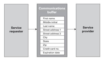
Figure 7.6 When we use a fixed communication area to connect two systems, we tightly couple the requester and provider. Changes to the interface—for example, an added country or a ninedigit ZIP code—can render the interface obsolete.
