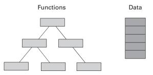
Figure 2.5 Structured programming calls for the separate creation and maintenance of major data structures and programs. Taking larger procedures and decomposing them into smaller ones control complexity but can make maintenance problematic. The famous Y2K bug thrived under conditions of structured programming.
