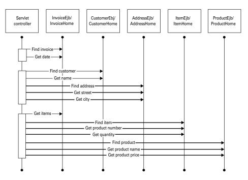
Figure 8.5 This sequence diagram graphically illustrates the round-tripping problem. We have a distributed interface between the controller and the EJB objects. The bold lines indicate places where we have significant looping. The UML sequence diagram is ideal for detecting round-tripping.
