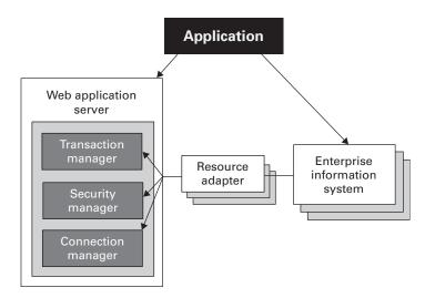
Figure 7.4 The J2EE common connector architecture uses vendor-provided adapters, operating through a common interface, to collaborate with the web application servers to provide transaction integrity, security, and efficient connection management. Connection pooling is included in the specification.
