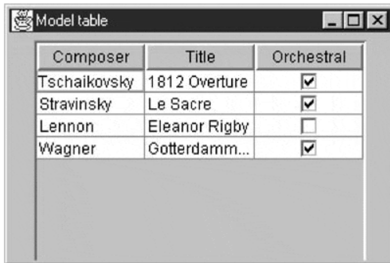
Figure 32.2. A JTable display using a data model that returns the data type of each column and controls the data display accordingly.
