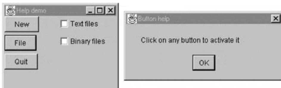
Figure 16.6. A simple help demonstration that pops up a different message, depending on which control is selected when the F1 key is pressed.
