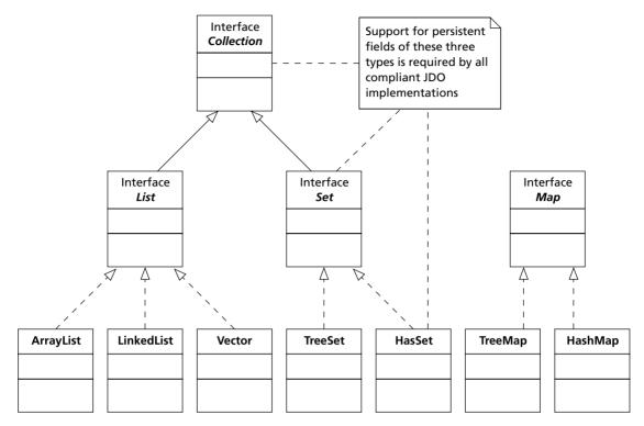
Figure 5.8 Simplified UML class diagram for the Java 2 Collections
