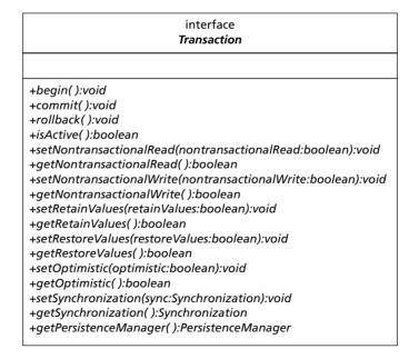
Figure 7.1 UML for Transaction interface
