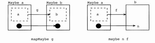
Figure 14.4 Error-handling functions.
