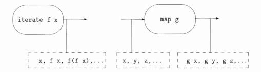
Figure 17.3 A generator and a transformer.
