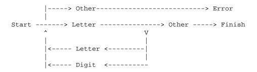
As you can see, this diagram shows how the logic flows as characters are read. Things begin, of course, in the start state, and end when a character other than an alphanumeric is found. If the first character is not alpha, an error occurs. Otherwise the machine will continue looping until the terminating delimiter is found.
