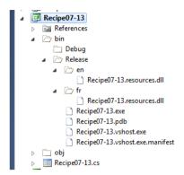
Figure 7-9. Satellite assembly structure
