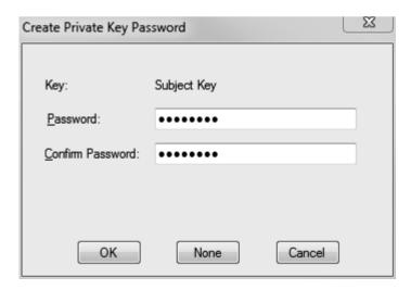
Figure 1-2. The Certificate Creation tool requests a password when creating file-based private keys.
