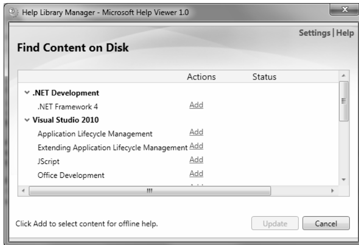
Figure 2-24. The Help Library Manager allows you to download a local copy of the .NET Framework 4.0 SDK Documentation
