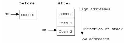
Before the items are pushed, SP points to (holds the address of) the previous item that was pushed. After two new words have been pushed, the stack pointer points to the second of these, and the first word pushed lies 'underneath' it.
