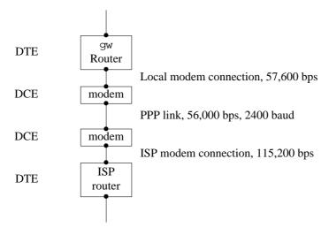
Figure 19-2: Network modem connection
