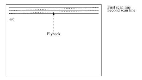
Figure 28-1: Scanning pattern on the monitor
