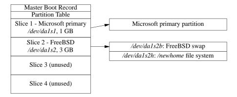
Figure 11-3: Partition table on second FreeBSD disk
