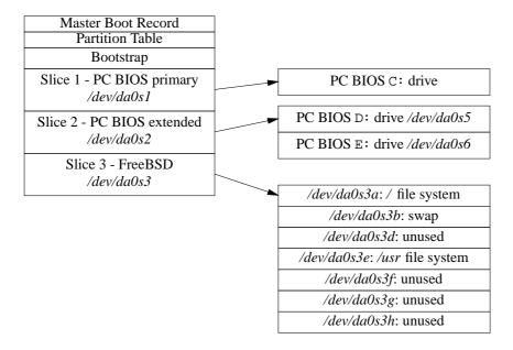
Figure 2-2: Partition table with FreeBSD file system
