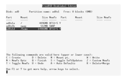
Figure 5-13: Completed partition allocation
