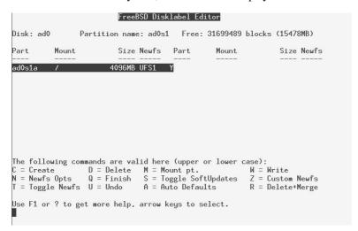
Figure 5-12: Allocated root file system
