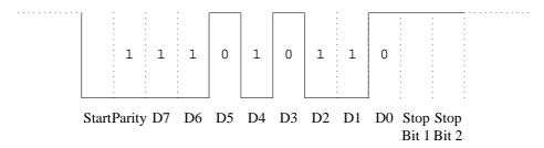
Figure 19-1: Asynchronous byte encoding
