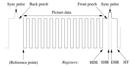
Figure 28-2: Scan line and register values
