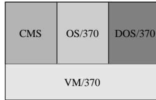
Figure 4.5 Virtual machine operating system VM/370.
