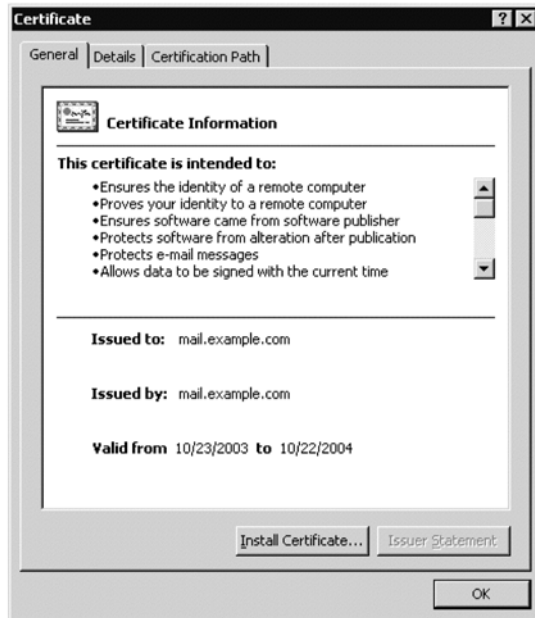
Figure 17-3: A successfully installed CA certificate on a Windows host
