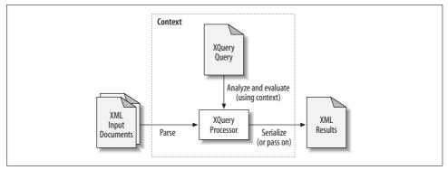
Figure 2-1. A Basic XQuery processor
