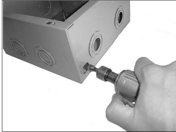
Figure 11.8 Keying a Hole for an N-Type Female Bulkhead
