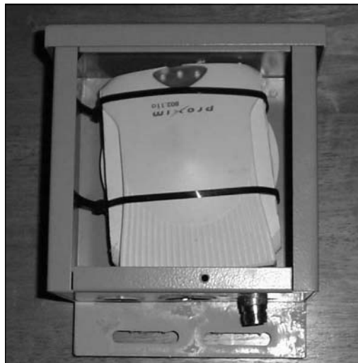
Figure 4.24 8571 Mounted in an Electrical Box
