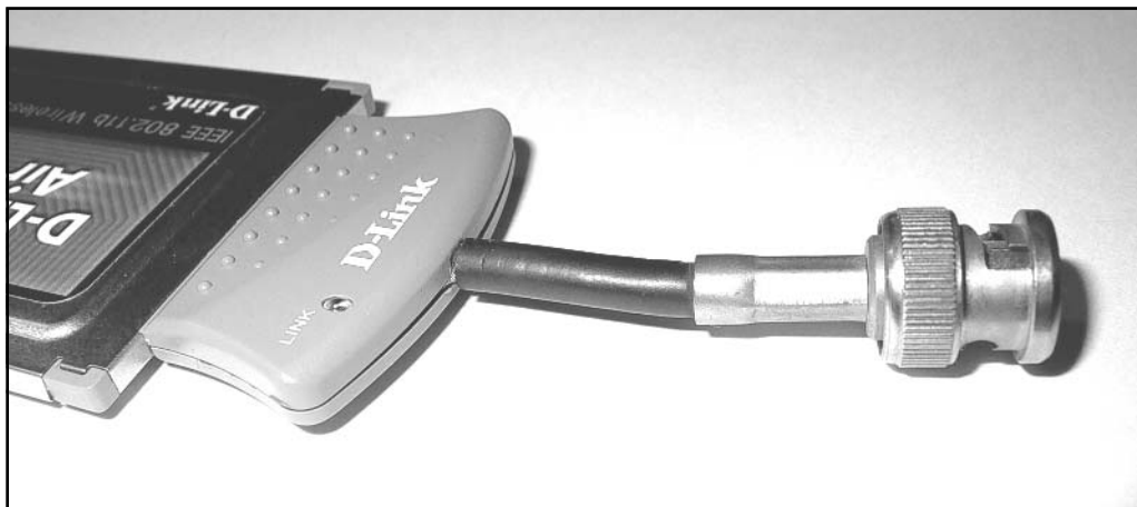
Figure A.11 The Finished Hack: D-Link DWL-650 with External Antenna Connector
