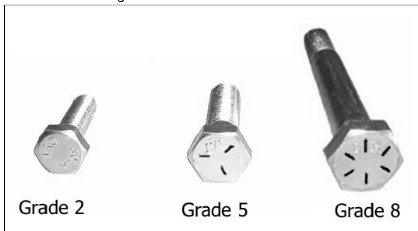
Figure 11.2 SAE Grade Markings on Bolt Heads
