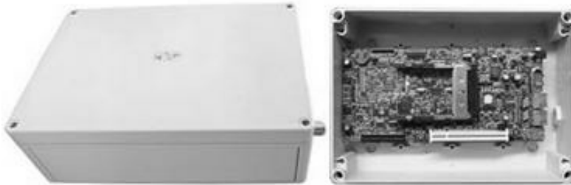
Figure 8.9 RouterBOARD 230 Outdoor Kit
