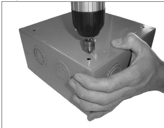
Figure 11.6 Removing Burrs with a Countersink Drill Bit
