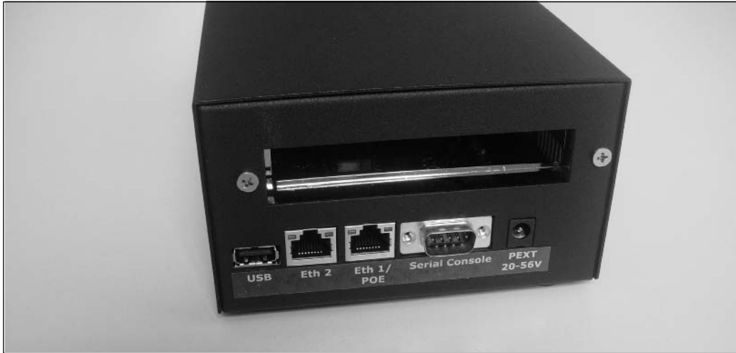
Figure 8.9 RouterBOARD 230 Outdoor Kit
