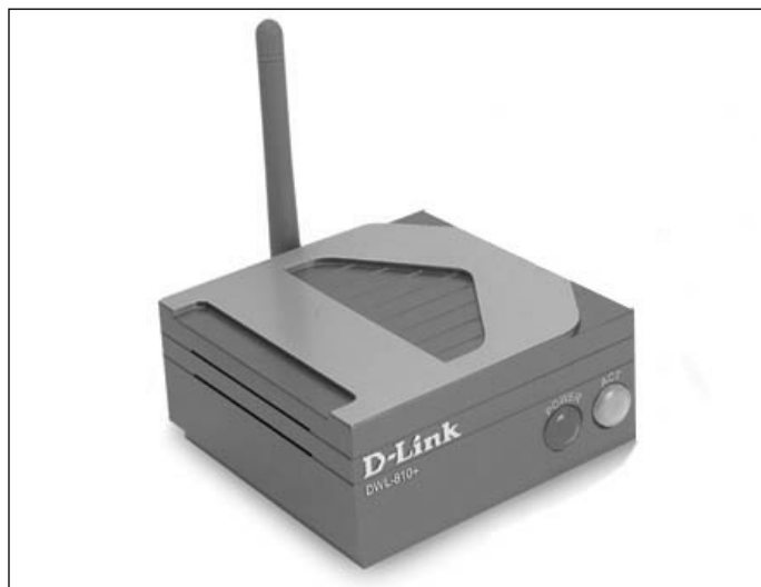
Figure 2.2 Enhanced 2.4 GHz Ethernet to Wireless Bridge
