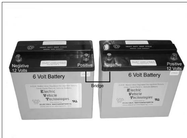
Figure. 12.11 Batteries Wired in a Series
