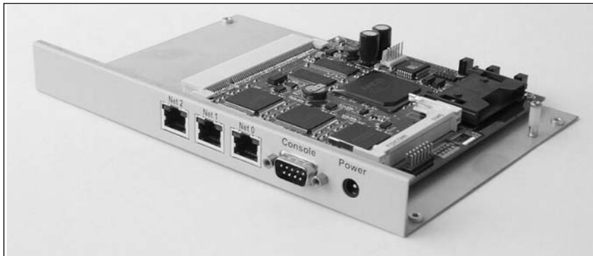
Figure 4.14 net4501 Without a Cover
