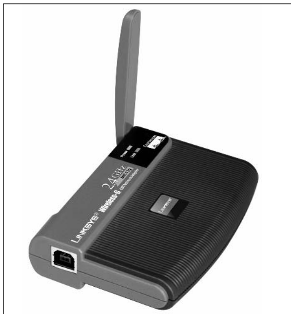
Figure 5.6 Another USB Adapter (pictured Linksys WUSB54G)
