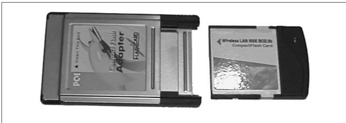
Figure 5.9 Another Compact Flash adapter w/ PCMCIA sled (pictured AmbiCom WL1100C-CF)
