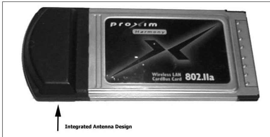
Figure 5.1 A typical PCMCIA card (pictured Proxim Harmony 802.11a card)
