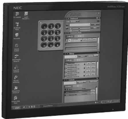
Figure 10-3: A soft phone running on a Windows PC.
