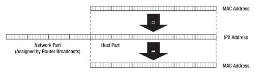
Figure 1-2. The IPX address and the Ethernet MAC address
