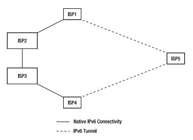
Figure 4-5. Native versus tunneled connectivity in IPv6
