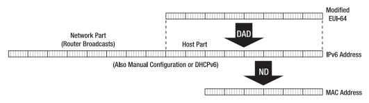
Figure 1-7. The IPv6 address, the EUI-64, and the Ethernet MAC address
