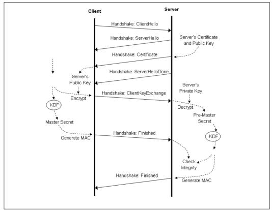
Figure 14.3 SSL Handshakes for Certificate and Key Exchange
