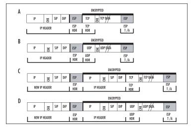
Figure 13.12 ESP Header: Transport Mode and Tunnel Mode
