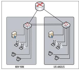
In Figure 13.3, dotted lines represent VLAN 2, solid lines represent VLAN 10, and dash-dot lines represent VLAN 100. The presence of the three lines that form a trunk between the top level switches should not be taken to indicate that there are three physical connections. In the network shown in Figure 13.3, broadcast traffic in the telephone subnet will not be seen by hosts in the workstation subnet.
