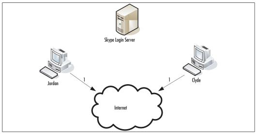
The users use TCP ports to connect to the Skype login server (2) via the Internet (see Figure 7.2). The connection is secured using 256-bit AES encryption. The symmetric AES keys that are negotiated between the server and client are handled using 1536- and 2048-bit RSA.
