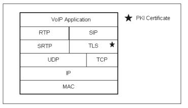
Figure 14.1 Layered Architecture of VoIP Security Protocol
