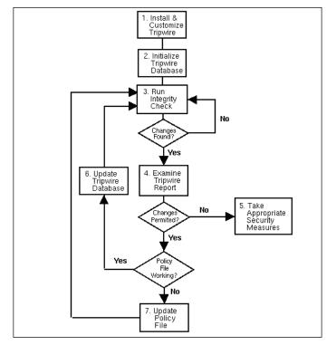
Figure 10.3 A Diagram of Tripwire Processes
