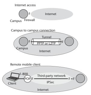
Figure 6.10 VPN basic connections.
