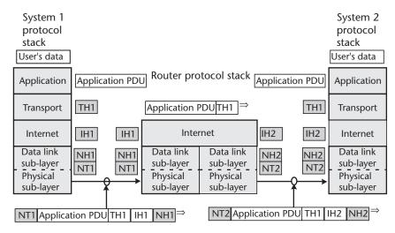
TH Transport Layer Header; IH Internet Layer Header; NH Network Interface Layer Header; NT Network Interface Layer Trailer
