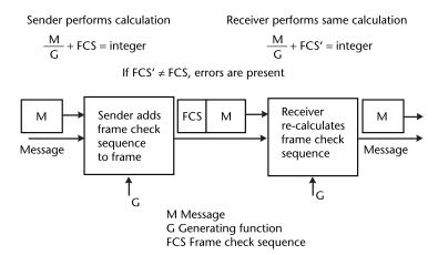
Figure A.10 Principle of cyclic redundancy check.
