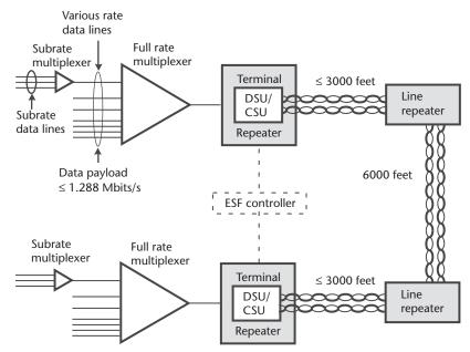
Figure 7.5 T-1 data-only configuration.
