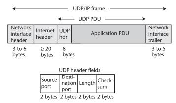
Figure 1.2 UDP header and UDP/IP frame.
