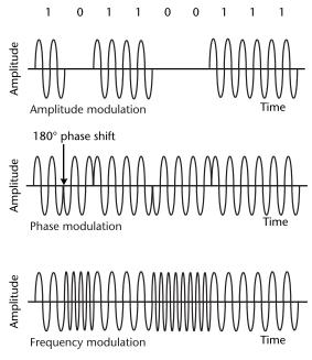
**Figure A.5** Amplitude, phase, and frequency keying.
