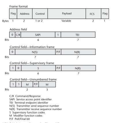
Figure 4.1 HDLC Link Access Protocol—Channel D.
