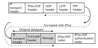
**Figure 6.8** L2TP encapsulation with privacy and authentication.
