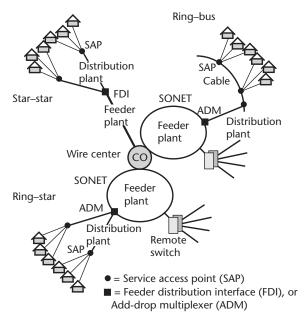
**Figure 8.2** Alternative architectures for loop plant.
