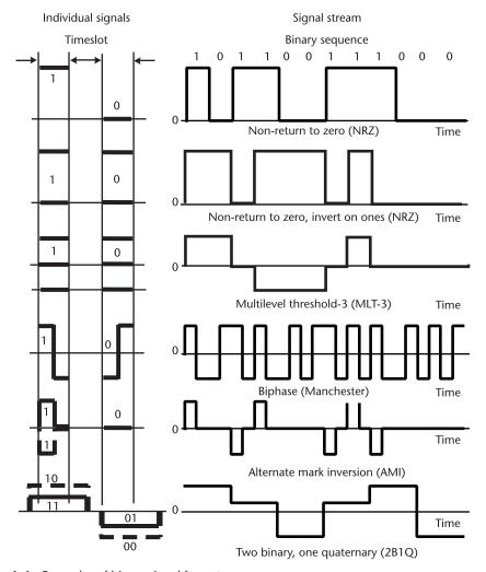
Figure A.4 Examples of binary signal formats.
