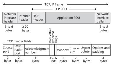
Figure 1.3 TCP header and TCP/IP frame.
