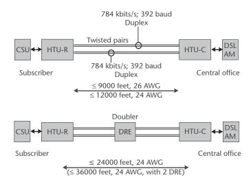
HTU-CHDSL Transceiver unit—central office HTU-RHDSL Transceiver unit—remote CSU Channel service unit DSLAM Digital subscriber line access multiplexer DREHDSL Range extender
