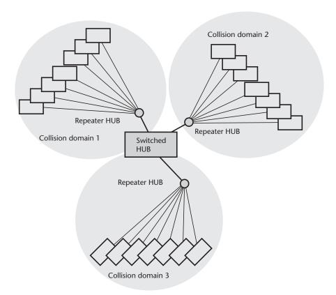
Figure 3.8 Use of switched hub to link Ethernets and separate collision domains.
