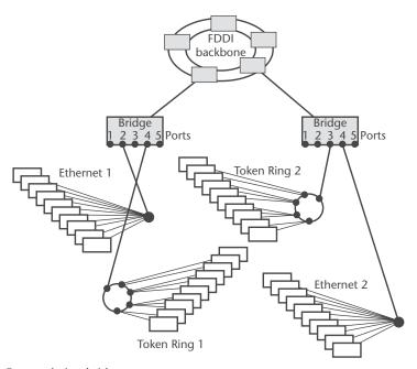
Figure 5.7 Encapsulating bridges.
