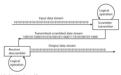
**Figure A.2** Principle of scrambling.
