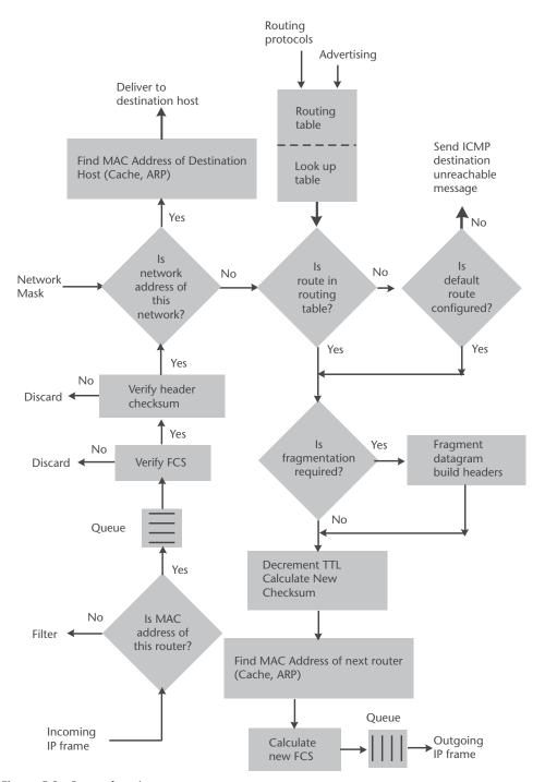
**Figure 5.9** Router functions.
