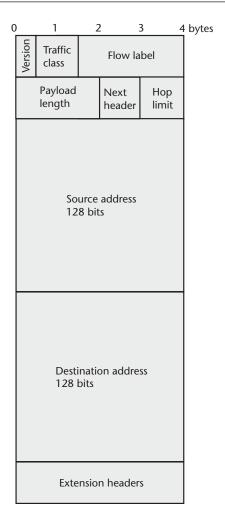
Figure 1.9 IPv6 header.
