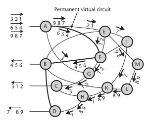
Frames 1, 2, and 3 are sent from A to C with distributed routing Frames 4, 5, and 6 are sent from A to B over a permanent virtual circuit Frames 7, 8, and 9 are sent from A to D using centralized routing
