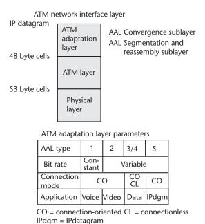
Figure 4.8 ATM protocol layers.
