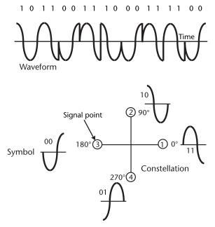
Figure A.6 Example of QAM to create a signal in which each symbol represents 2 bits.
