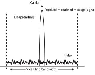
**Figure A.8** Illustrating the spreading of a message signal and the despreading of a spread spectrum signal to yield the message signal and mitigate noise.
