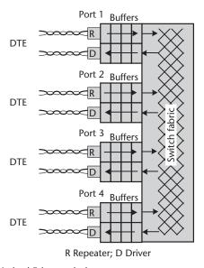
Figure 3.7 Principle of switched Ethernet hub.
