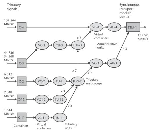
Figure 7.13 Tributary multiplexing scheme to create STM-1 frame.
