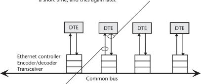
Monitors receive channel for frames addressed to station, for periods of no activity, and to detect collisions when sending frames
