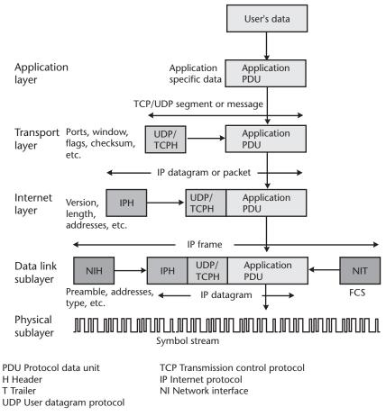
Figure 2.4 Formation of IP datagram and IP frame.
