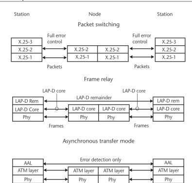
Figure 4.6 Protocol stacks for packet switching, frame relay, and ATM.
