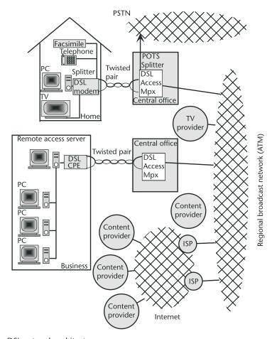
Figure 8.3 DSL network architecture.
