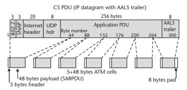
Figure 4.9 Division of CS PDU (IP datagram with AAL 5 trailer) into ATM cells.
