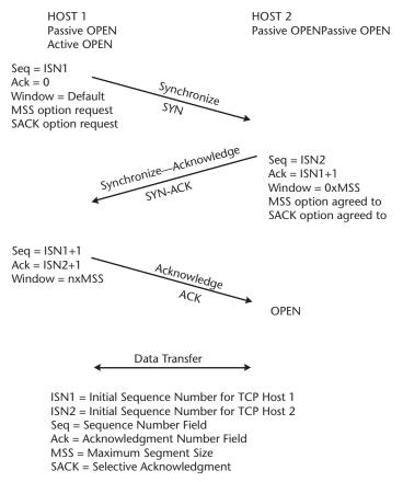
Figure 1.4 TCP connection establishment procedure.
