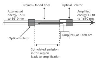
Figure 7.9 Principle of Erbium-doped fiber amplifier.
