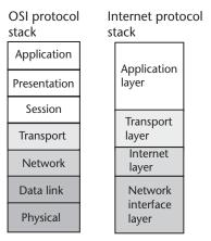
Figure 2.3 Comparison of OSI and Internet Protocol stacks.
