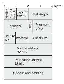
Figure 1.7 IPv4 header.
