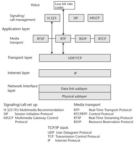
**Figure 8.6** TCP/IP stack with VoIP protocols.
