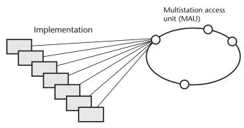
Figure 3.9 Principle of Token Ring LAN.
