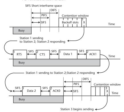
Figure 7.17 Illustrating collision avoidance.
