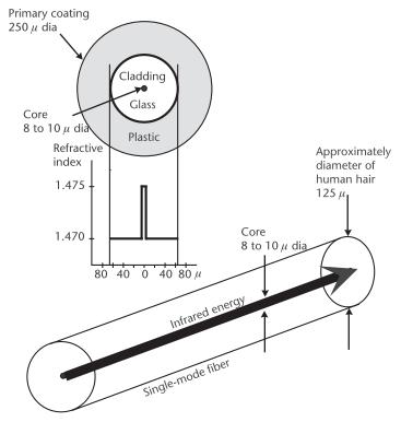
Figure 7.8 Single-mode optical fiber.
