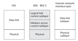
Logical Link Control Sublayer: defines format and functions of PDUs passed between SAPs (service access points) in source and destination
