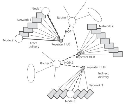
Figure 5.8 Direct and indirect delivery.
