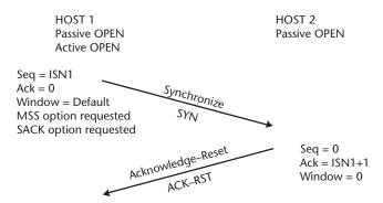
**Figure 1.5** TCP connection reset procedure.
