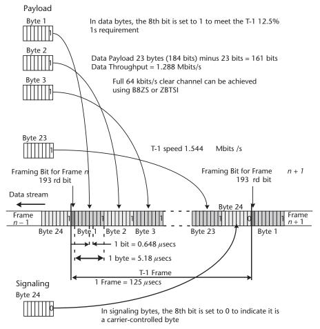
Figure 7.6 T-1 data frame format.
