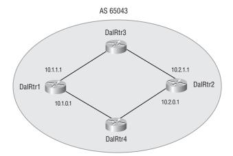
The *update-source* configuration is typically used only for IBGP connections. This is because by default EBGP connections must be directly connected. The time to live (TTL) of all EBGP packets is 1. A loopback interface is not directly connected as the packet must pass through the physical interface and be routed to the loopback.
