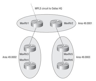
Start with the basic command set to get IS-IS running on a router. The first command simply starts the IS-IS protocol. The only option is the area tag, which is just like the process
