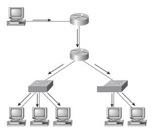
FIGURE 8.2 Sending Multicast Traffic to Multiple Hosts
