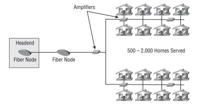
The actual bandwidth for Internet service data over a CATV line can be up to about 27 Mbps on the download path to the subscriber, with about 2.5 Mbps of bandwidth on the upload path. Depending on the cable network architecture, cable operator provisioning practices, and traffic load, an individual subscriber can typically get an access speed from 256 kbps to 6 Mbps.
