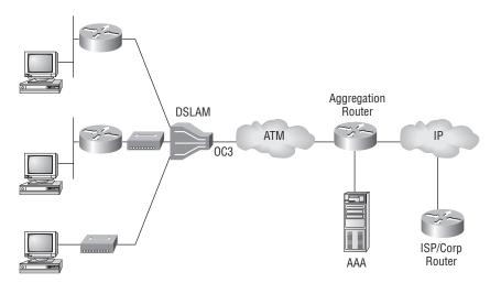
In the PPPoE architecture, the PPPoE client connects to the ADSL service. The PPPoE client first encapsulates the end user data into a PPP frame, and then the PPP frame is further encapsulated inside an Ethernet frame. The IP address allocation process for the PPPoE client is same as PPP in dial mode.
