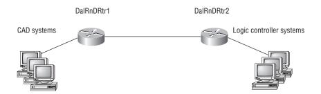
If you use autoconfiguration to address your subnets, each of the clients and devices on a subnet will get an address, but the address is a link-local address. That means that the CAD systems the RnD guys have on one subnet will be able to talk, but the logic controller systems would not be able to communicate with CAD systems. Autoconfiguration is very useful for getting basic connectivity to systems, but not for complete connectivity.
