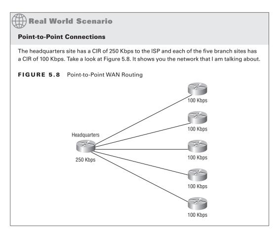
Before we even get to the routing portion of this example, let's look at the first thing that would have probably been done in this situation. If the CIR bandwidths were to be configured on the interfaces, in this case you would end up with an aggregation problem. If each of the sites were to send their maximum 100 Kbps to the HQ site at the same time, the HQ side of the connection would be overloaded. For this reason, the bandwidth at the remote site would be set artificially low to 50 Kbps.
