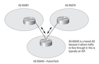
BGP does not work in the same manner as IGPs. Because the designers of BGP could not guarantee that an AS would run BGP on all routers, a method had to be developed to ensure that IBGP speakers could pass updates to one another while ensuring that no routing loops would exist.
