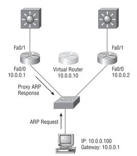
With proxy ARP, the host device sends traffic as if the destination device were located on its own network segment. If the router that responded to the ARP request fails, the source host continues to send packets for that destination to the same MAC address, but since that is to a failed router, the packets will be discarded.
