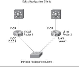
To accommodate the traffic, two virtual router groups are configured. For virtual router 1, PortRtr1 is the owner of IP address 10.0.0.1 and is therefore the master virtual router for clients configured with that default gateway address. PortRtr2 is the backup virtual router to PortRtr1.
