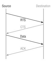
CSMA/CA is also called a Request to Send, Clear to Send (RTS/CTS) because of the way that hosts must communicate with the AP. For every packet sent, an RTS/CTS and acknowledgment must be received; because of this rather cumbersome process, it's kind of hard to believe it all actually works!
