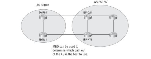
Unlike local preference, the MED is exchanged between autonomous systems. The MED is sent to EBGP peers; those routers propagate the MED within their AS, and the routers within the AS use the MED but do not pass it on to the next AS. When the same update is passed on to another AS, the metric is set back to the default of 0.
