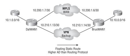
For this example, the only routing protocol FutureTech is running on the network is EIGRP, so you can make the distance anything above 90. Let's make it 95 for the example. You need to tell the DalWAN1 router what the redundant path to get to all the destination subnets in Brussels is. The subnets that exist in Brussels, as you have seen from the previous
