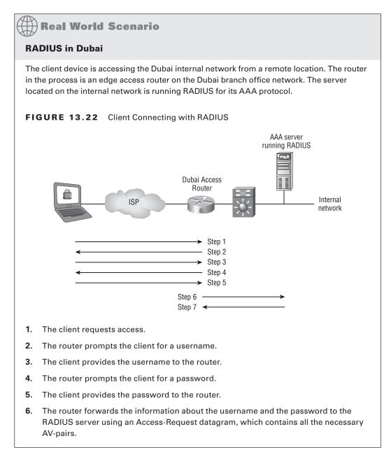
7. If the user information is correct, the server responds with an Access-Accept datagram. The Access-Accept message also contains authorization parameters in the form of AV-pairs, such as the IP address to be assigned, and so on.
