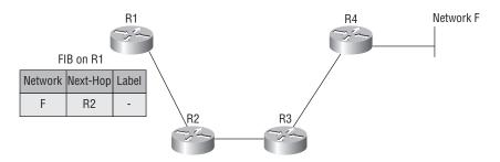
To begin, all of the routers exchange updates and build their routing tables. Now, as far as MPLS is concerned, it doesn't matter what routing protocol they are running. The routing protocol is running and all of the routers have up-to-date routing tables.
