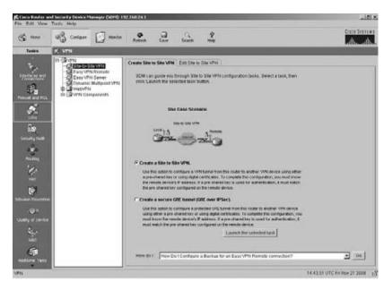
FIGURE 12.6 Cisco Router and Security Device Manager Create Site to Site VPN Tab
