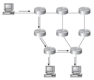
Packets are forwarded through the SPT using the source and group address pair. Because of this the routes are written like with this notation (S, G) (pronounced "S comma G"), where S is the IP address of the source and G is the multicast group address. The multicast route entries appear in the multicast tables and look like this:
