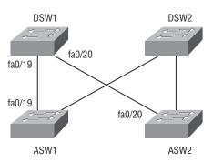
The configurations in this section give you flexibility in the type of switches that you can use. If you have the 3560 switches that I mentioned in the test network setup, then you are good to go. For this section, if you have 2950s, 2960s, or 3550s, you also will be just fine. When you get down to the inter-VLAN routing configuration, you will have to have at least one 3550 or 3560 to use as a distribution layer switch.
