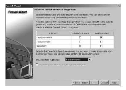
**FIGURE 15.20** Cisco Router and Security Device Manager Advanced Firewall DMZ Service Configuration
