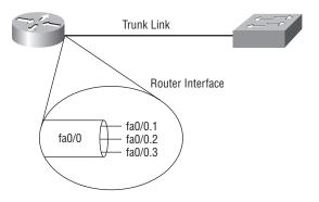
The routing table on the router will show directly connected subnets that are associated with each of the VLANs. They are just configured on the router's subinterfaces. The router must still learn routes to networks that are not directly connected via a dynamic routing protocol.
