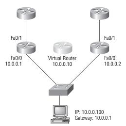
I am sure that you are asking, "Is there another way to use the other router?" The answer is complicated. There is feature that is enabled by default on Cisco routers called Proxy Address Resolution Protocol (Proxy ARP). Proxy ARP enables hosts, which have no knowledge of routing options, to obtain the MAC address of a gateway router that can forward packets off of the local subnet for them.
