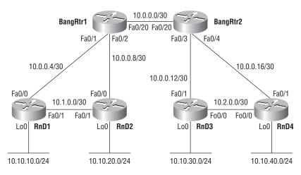
Let's start with the core routers. I want to enable OSPF on each of the interfaces.
