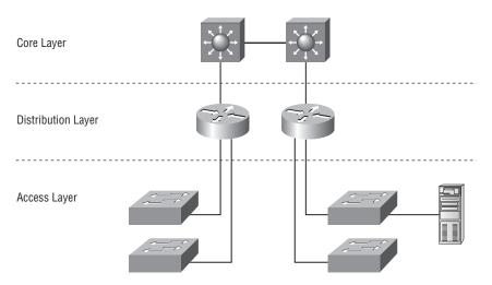
FIGURE 1.1 Three-layer hierarchical design model
