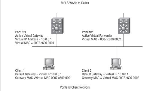
Like HSRP, GLBP can be configured to track interfaces. Take a look at Figure 10.14. If the WAN link from router PortRtr1 is lost, GLBP detects the failure because interface tracking is configured on PortRtr1. The job of forwarding packets for virtual MAC address 0007.c600.0001 will be taken over by the secondary virtual forwarder for the MAC, router PortRtr2. Therefore, the client sees no disruption of service nor does the client need to resolve a new MAC address for the default gateway.
