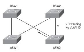
Normally, broadcast traffic would be carried to all the switches for a VLAN, if that VLAN existed on all of the switches. But, what if one of the access switches didn't have any ports in a given VLAN? There would be no use in sending broadcast traffic to that switch because it has no hosts to send the broadcast to.
