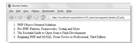
**Figure 7-12.** A combination of LimitIterator and AppendIterator makes it possible to select the first two from each source.
