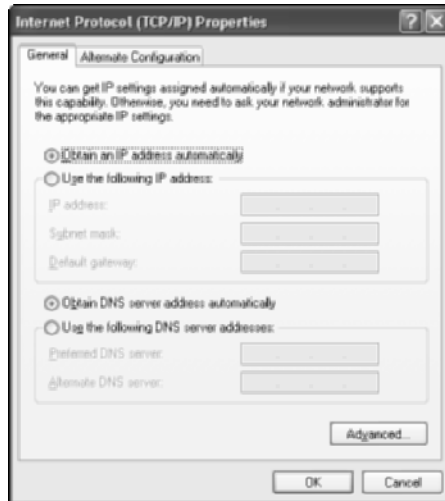
Figure 3-8: Configuring a Windows client to use DHCP.
