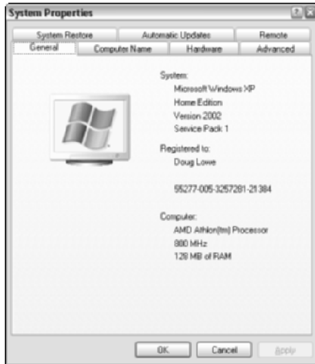
Figure 1-2: The System Properties dialog box for a computer running Windows XP Home Edition with 128MB of RAM.
