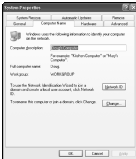
Figure 4-6: The Computer Name tab of the System Properties dialog box (Windows XP).
