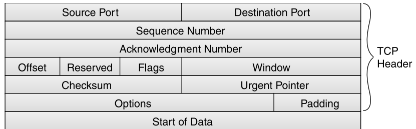
FIGURE 4.2 A datagram with its TCP header
