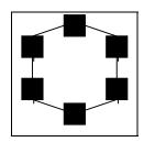
**Ring** - All computers are connected via a single cable. However, the ends are not terminated and the cable forms a full loop connecting the last computer to the first computer.
