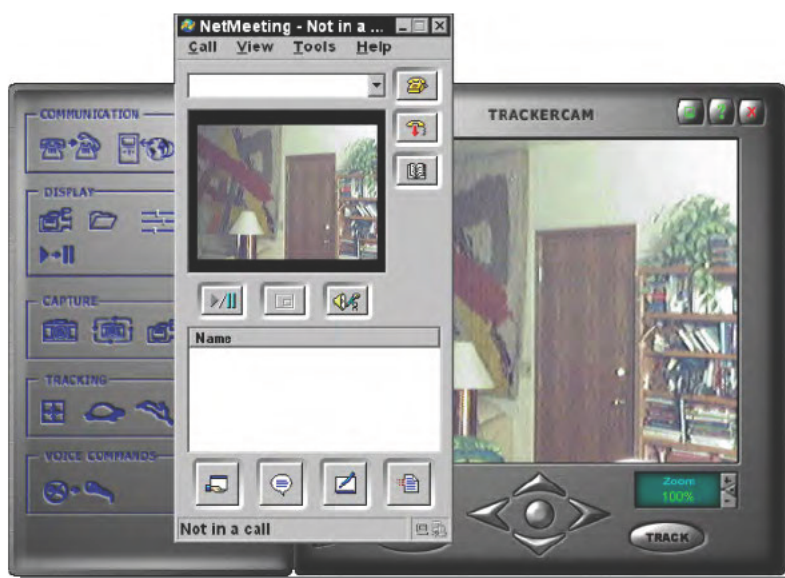
FIGURE 6-12: Configure NetMeeting to use the TrackerCam Capture camera and you'll have motion tracking from within NetMeeting.
