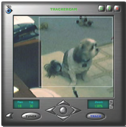
FIGURE 6-10: A bounding box in the camera view shows the area TrackerCam identified as containing motion.
