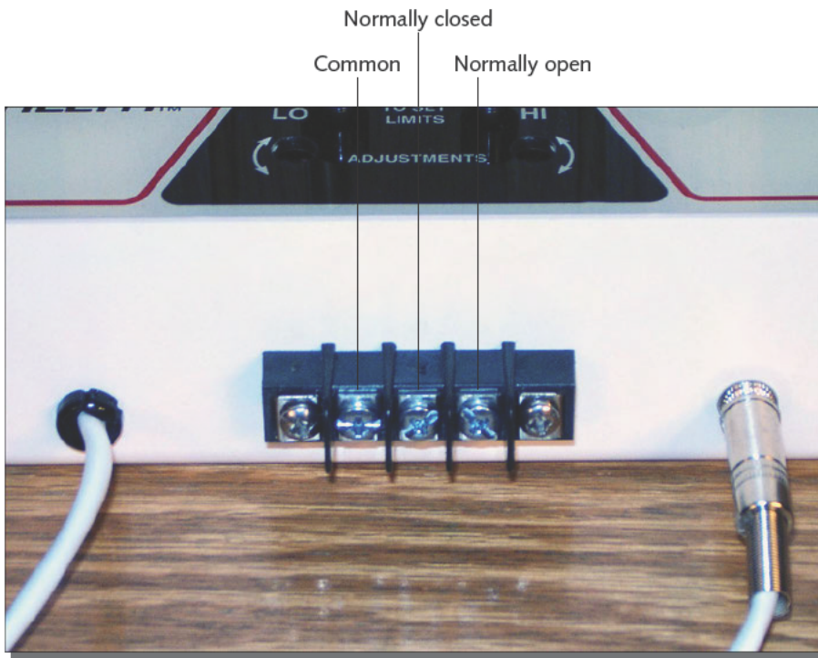
FIGURE 7-5: DTA-1 contact terminal strip
