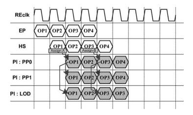
Figure 7.21 Horizontal setup: pipeline timing
