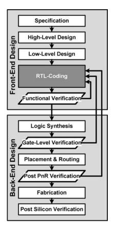
Figure A.1 Typical design flow
