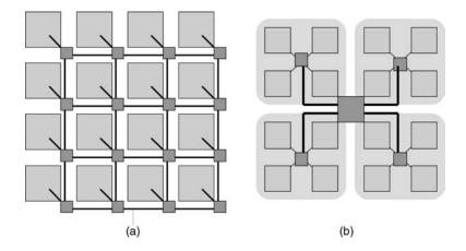
Figure 2.23 Topologies: (a) mesh, and (b) hierarchical star
