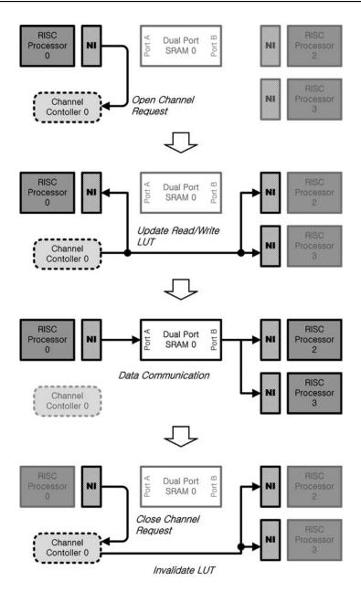
Figure 2.37 Important steps of the MC-NoC operation
