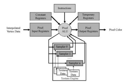
Figure 3.16 Pixel shader model
