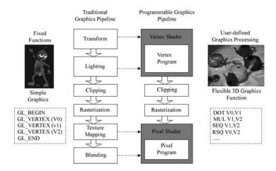
Figure 3.14 Programmable 3D graphics pipeline
