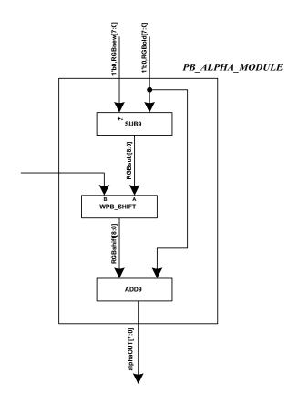
Figure 7.38 Datapath #2: PB\_ALPHA\_MODULE
