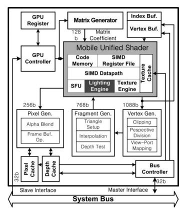
Figure 6.15 Block diagram of RAMP-VII
