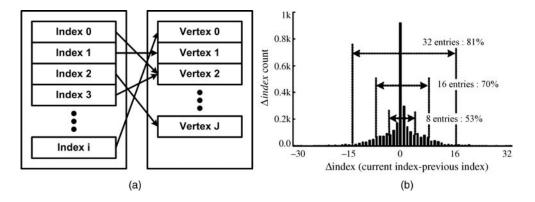
Figure 5.13 Characteristics of the indexed vertex: (a) vertex ordering, and (b) coverage of the  $\Delta$  index
