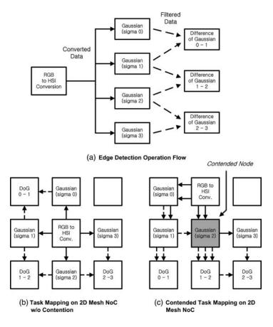
Figure 2.39 Mapping of edge detection task into conventional mesh NoC
