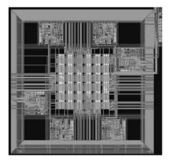
Figure 2.19 Switch layout diagram of  $6 \times 6$  and phit width of 10 bits/link
