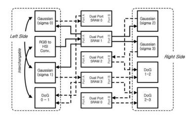
Figure 2.40 Mapping of edge detection task on MC-NoC
