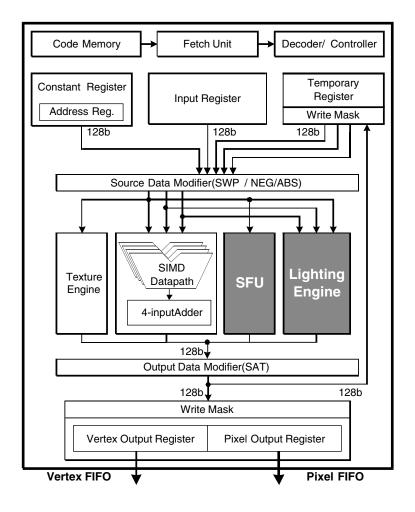
Figure 6.16 Mobile unified shader
