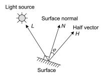
Figure 3.5 Geometry for specular lighting
