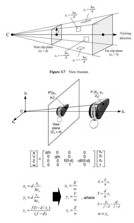
Figure 3.8 Perspective transformation and its matrix
