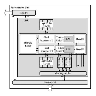
Figure 7.2 Block diagram
