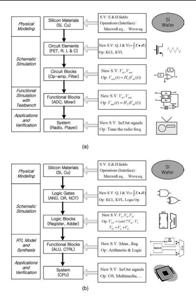
Figure 2.5 Applying (a) analog and (b) digital designs
