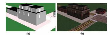
Figure 3.13 Texture mapping effects: (a) flat shaded image, and (b) texture-mapped image
