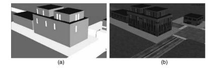
Figure 3.13 Texture mapping effects: (a) flat shaded image, and (b) texture-mapped image
