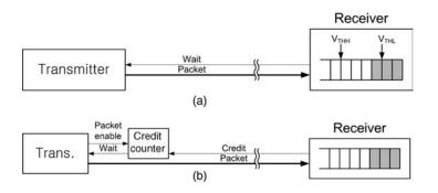
Figure 2.13 Flow control schemes: (a) back pressure, and (b) credit-based flow control
