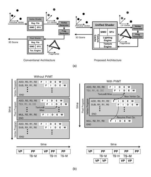
Figure 5.18 Pixel-vertex multi-threading: (a) data flow diagram, and (b) pixel-vertex multi-threading
