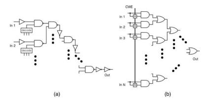
Figure 2.18 Circuits for crossbar switch: (a) tree of NAND invertors, and (b) pre-programmed
