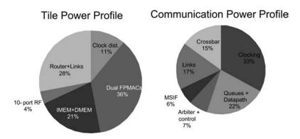
Figure 2.35 Power breakdown of a tile and NoC building blocks
