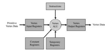
Figure 3.15 Vertex shader model
