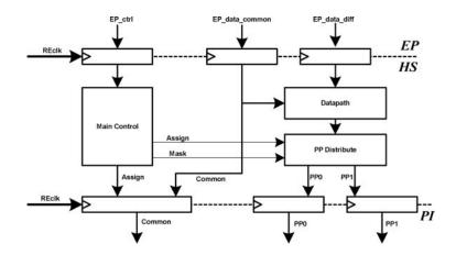
Figure 7.18 PP control scheme: block diagram
