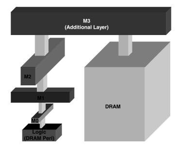
Figure 4.4 Embedded DRAM vs. DRAM-based SoC process technology
