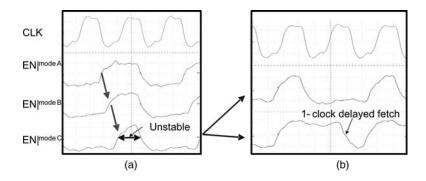
Figure 2.29 (a) EN signal variation according to the modes, and (b) unstable EN signal fetching
