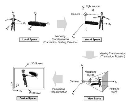
Figure 3.2 Spaces and coordinate systems in 3D graphics
