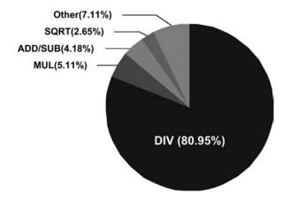
Figure 5.3 Percentage of processing time of the 3D graphics rendering pipeline
