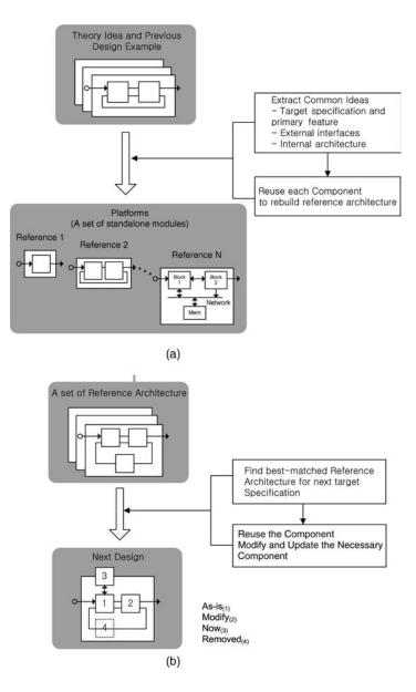
Figure 2.1 (a) Platform and (b) set-based design
