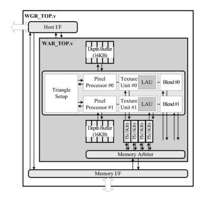
Figure 7.7 Module block diagram
