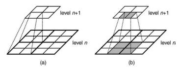
Figure 5.11 Mipmap pyramid: (a) conventional approach, and (b) bilinear-average mipmap
