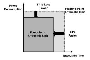
Figure 6.8 Energy saving by fixed-point arithmetic, measured during transformation operations
