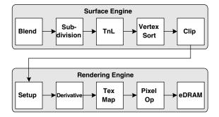
Figure 6.27 Sony PSP<sup>™</sup> 3D graphics pipeline
