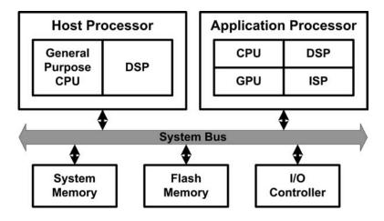
Figure 1.4 Embedded processors and system architecture
