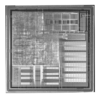
Figure 6.3 RAMP-IV chip micro-photo
