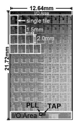
Figure 2.31 Intel's teraflop 80-core NoC chip. The Intel logo is a registered trademark of Intel Corporation
