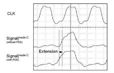
Figure 2.30 EN signal expansion using programmable delay synchronizer
