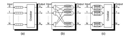
Figure 2.12 Queuing schemes: (a) input queuing, (b) output queuing, and (c) virtual output queuing
