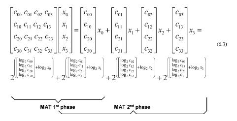
Taking note that the coefficients of a geometry transformation matrix are fixed during processing of a 3D object, these can be pre-converted into the logarithmic domain and be regarded as constants during the processing. Therefore, the required number of LOGCs for matrix–vector multiplication (MAT) can be reduced from twenty
