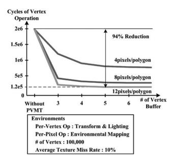
Figure 5.19 Efficiency of PVMT
