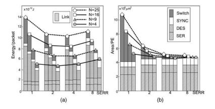
Figure 2.27 (a) Energy and (b) area of NoC according to SERR
