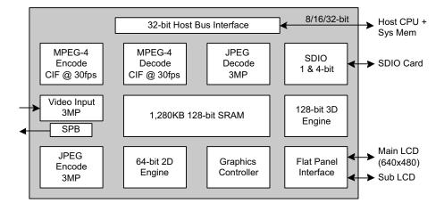
Figure 6.22 Block diagram of the nVidia SC10
