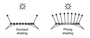
Figure 3.11 Shading schemes
