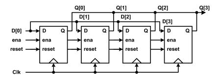
Figure A.9 Four-bit flip-flop
