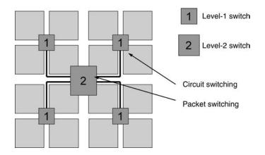
Figure 2.25 Adaptive switching method
