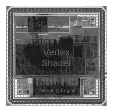
Figure 6.14 RAMP-VI chip micrograph
