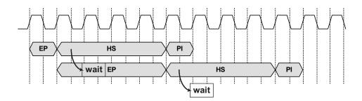
Figure 7.19 PP control scheme: pipeline timing
