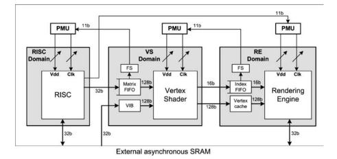
Figure 6.10 Proposed handheld GPU
