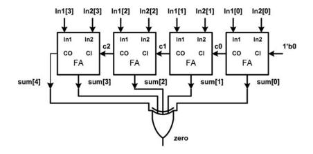
Figure A.10 Four-bit adder with zero detection
