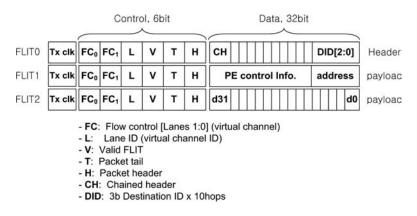
Figure 2.33 Packet format and protocols
