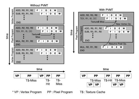
Figure 6.20 Pixel-vertex multi-threading
