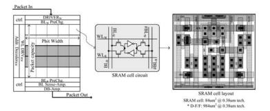
Figure 2.16 SRAM-based queue
