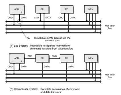
Figure 2.9 Bus and coprocessor
