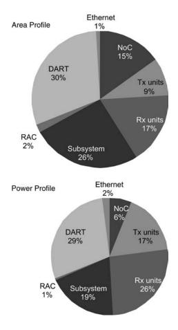
Figure 2.43 Area and power profile of the FAUST chip
