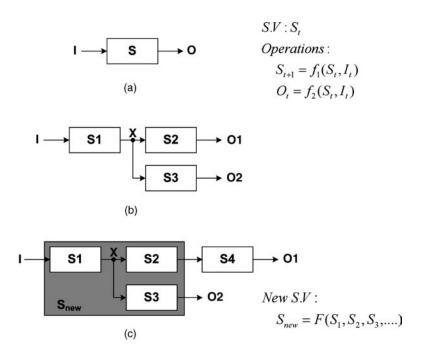
**Figure 2.3** Modeling and design methodology: (a) modeling, (b) modular design, and (c) hierarchical design
