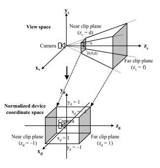
Figure 3.9 Normalized device coordinate space
