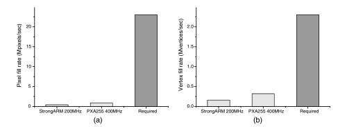
Figure 4.2 Performance graphs: (a) pixel fill rate, and (b) vertex fill rate
