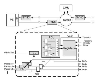
Figure 2.28 Programmable delay synchronizer
