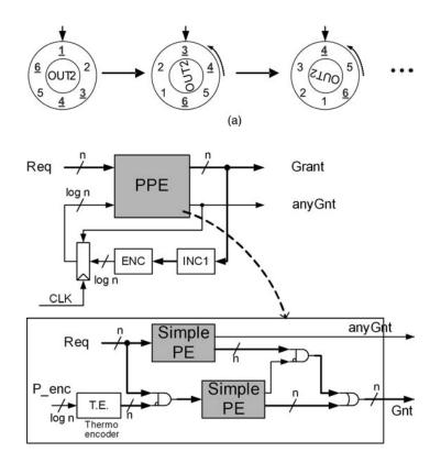
Figure 2.20 (a) Round-robin algorithm, and (b) round-robin algorithm circuits with two priority encoders
