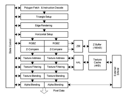
Figure 7.8 Pipeline architecture
