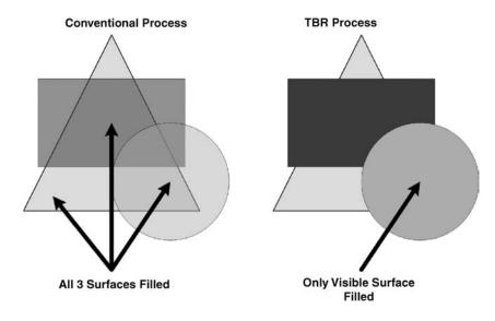
Figure 5.9 Tile-based rendering (HSR)
