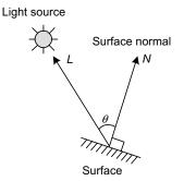
Figure 3.4 Geometry for diffuse lighting
