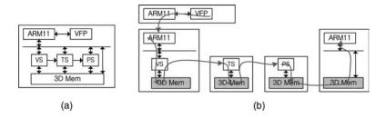
Figure 2.4 Example of use-case analysis: (a) block diagram, and (b) use-case analysis of a game
