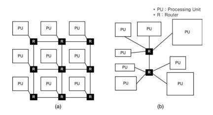
Figure 2.10 Two types of SoC: (a) homogeneous, and (b) heterogeneous
