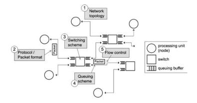
Figure 2.11 Basic design parameters of NoC
