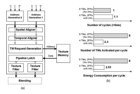
Figure 5.7 Address alignment logic: (a) block diagram, and (b) energy efficiency
