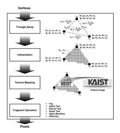
Figure 5.1 Simple rendering pipeline
