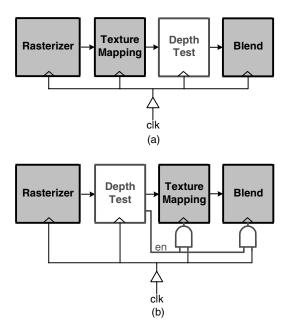
Figure 4.5 Depth reordering: (a) conventional pipeline, and (b) proposed pipeline
