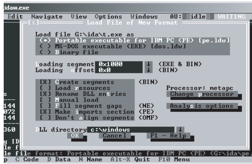
Figure 6-3: IDA executable file format box
