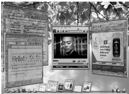
Figure 3-5: This view of Project Looking Glass shows word processing, video, and web browser windows in 3D. You can interact with existing 2D applications while learning how to use new 3D applications.
