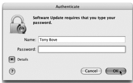
Figure 7-4: If some attachment or program tries to install anything with Mac OS X, it asks you for a password first. You can, of course, cancel it.
