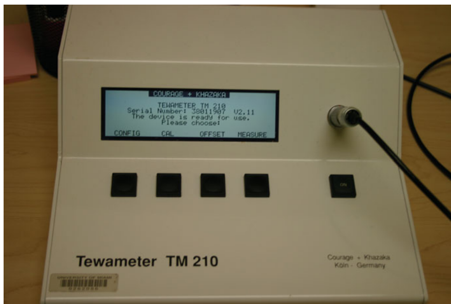
▲ FIGURE 38-1 The Tewameter is a brand of device similar to an evaporimeter.
