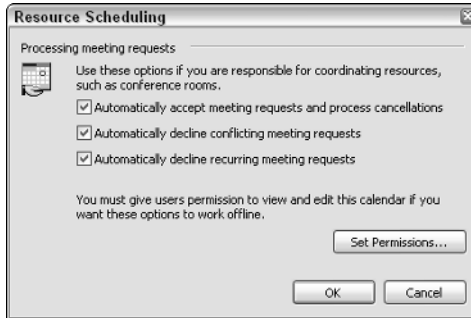
Figure 12-6: The Resource Scheduling dialog box lets you answer the request auto- matically.
