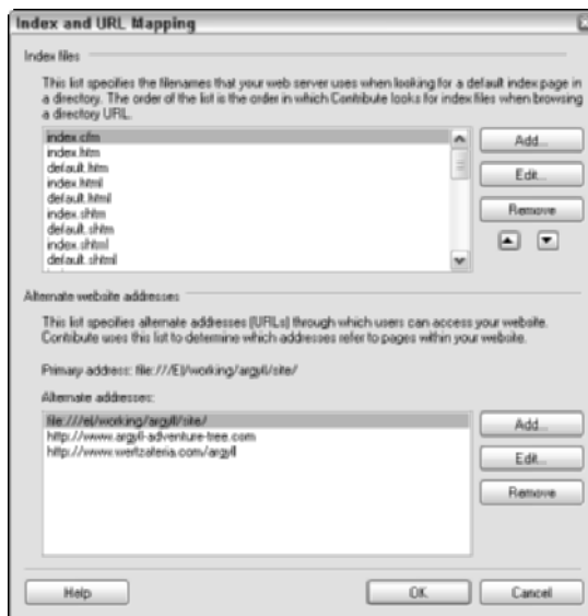
Figure 3-5: Contribute looks for pages on the server in the order in which the filenames appear in the Index files list.
