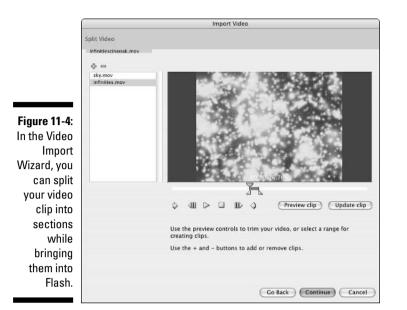
9. To change the beginning frame of a video clip, drag the leftmost triangle below the scrubber bar, or move the playhead to the desired frame and click the In button to set the new beginning frame. To change the ending frame of a video clip, drag the rightmost triangle below the scrubber bar, or move the playhead to the desired frame and click the Out button, to set the new ending frame.
