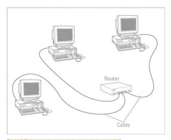
Figure 1-8: Each computer is connected to its own port in the router or hub.
