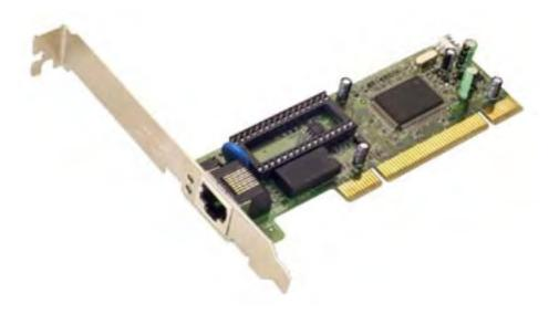
Figure 1-2: U.S. Robotics PCI network card.
