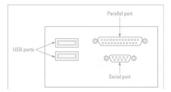
Figure 1-6: USB ports are identical in every computer.
