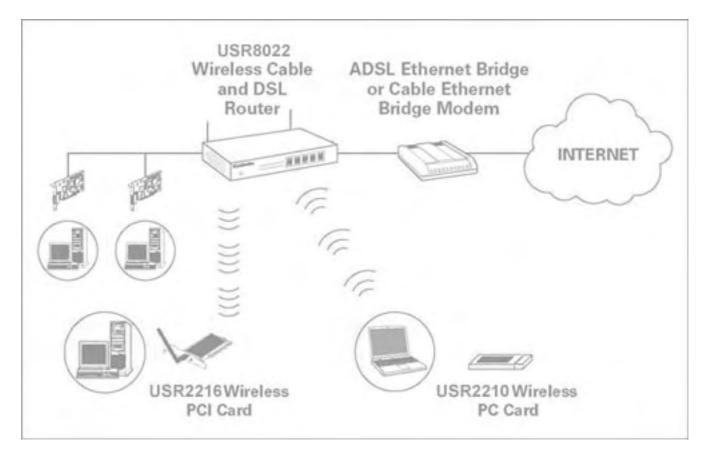
Figure 3-1: How a U.S. Robotics Model 8022 broadband router and an Internet connection all work together.
