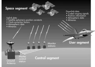
Figure 3-1: GPS is composed of satellites, ground stations, and receivers.
