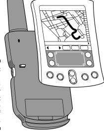
Figure 6-2: A Navman GPS receiver sleeve that slides on to the back of a PDA.
