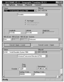
Figure 11-6: GeoTrans converts coordinates to another format.
