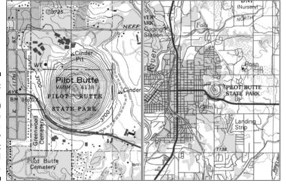
Figure 2-9: 1:24,000 and 1:100,000 scale topographic maps show different details and areas.
