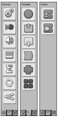
Figure 5.13 Programming blocks are accessed through one of three tabs on the Programming palette.
