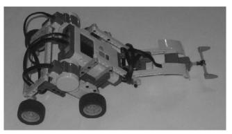
Figure 11.1 Detector Bot uses a touch sensor to determine when it has found its target.
