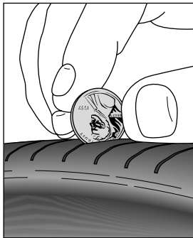
Figure 5-1: The penny test — this tire fails.
