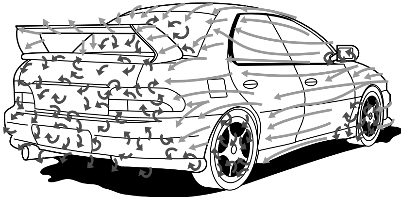
Figure 8-1: Airflow and the WRX: Why a tall wing is good.
