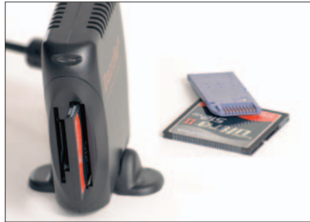
Figure 1-3: Card readers are the fastest, safest way to download images to your computer.
