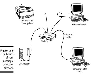
The wireless setup works the same as the wire-based setup. The difference is that in Figure 12-1, there would be no wires between the switch and the two computers and printer.
