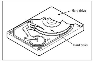
Figure 7-1: A run-ofthe-mill hard disk drive.
