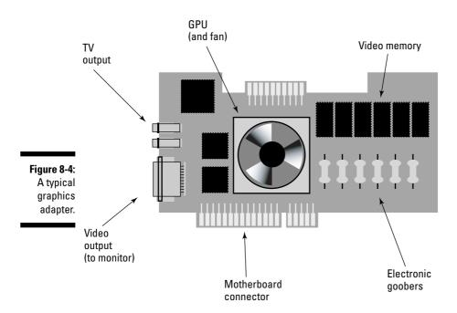
Several yardsticks measure graphics cards. The most important is whether the graphics adapter is a separate card or piece of circuitry, or whether the graphics circuitry is simply part of the chipset on the motherboard. Either way, the two values by which the graphics adapter is judged is how much video RAM it can access and whether it has any high-end functions, such as 3D ability or its own graphics processing unit (GPU).
