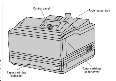
Figure 24-1: A chunky type of laser printer.
