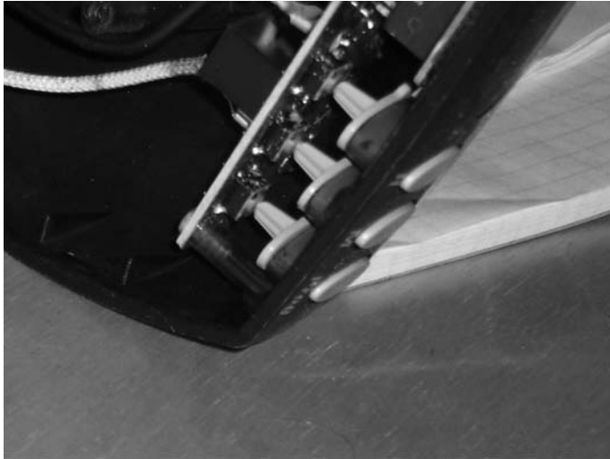
Figure 5.13: PCB switches in a cheap coffeemaker
