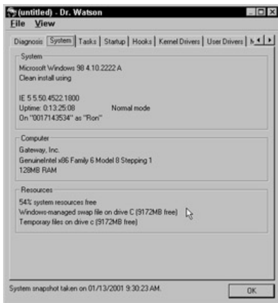
Figure 20-8: Dr. Watson is a Windows software diagnostic tool that can help you isolate the cause of General Protection Faults.
