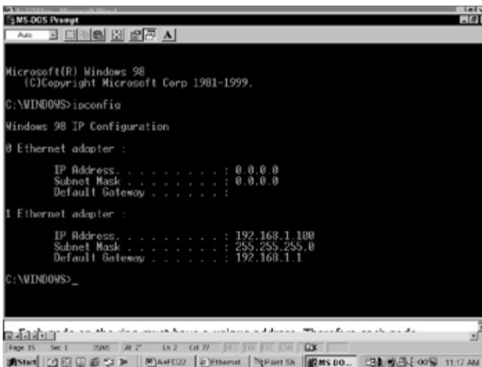
Figure 22-3: The IPCONFIG command is used to display the IP address configuration of a PC.
