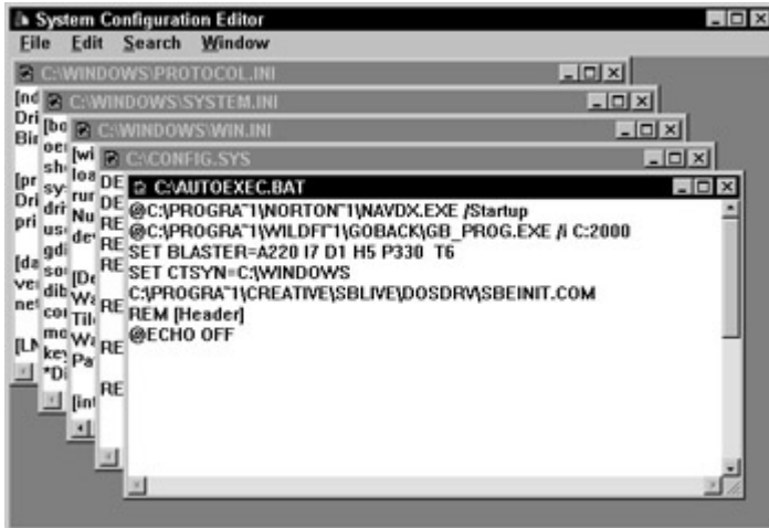
Figure 20-6: The SYSEDIT windows contain initialization and system files for viewing or editing.
