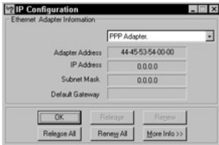
Figure 22-2: The WINIPCFG command can be used to display the MAC (Adapter) address of a PC's NIC.
