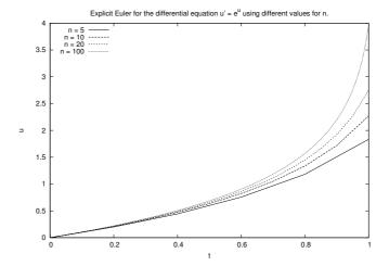
**Fig. B.2** Explicit Euler for the differential equation  $u' = e^u$  using different values for n.
