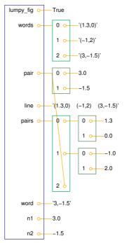
Fig. 6.3 Illustration of the variables in the read\_pairs.py program after the first pass in the loop over words in the first line of the data file.
