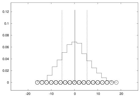
**Fig. 8.6** Particle positions (circles), histogram (piecewise constant curve), and vertical lines indicating the mean value and the standard deviation from the mean after a one-dimensional random walk of 2000 particles for 30 steps.
