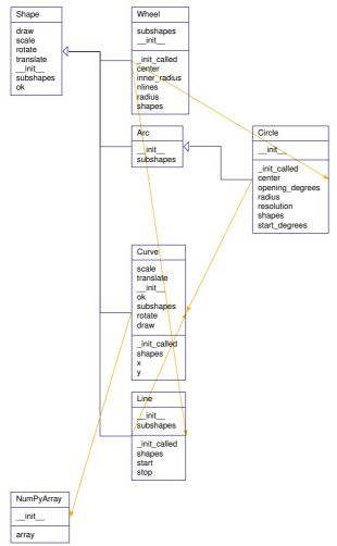
Fig. 9.13 This is a variant of Figure 9.12 where we display how class Wheel relates to other classes in the shapes hierarchy. Wheel is a Shape, like Arc, Line, and Curve, but Wheel contains Circle and Line objects, while the Circle and Line objects have a Curve, which has a NumPyArray. We also see that Circle is a subclass of Arc.
