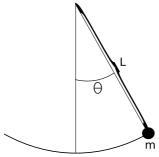
**Fig. B.4** A pendulum with m = mass,  $L = \text{length of massless rod and } \theta = \theta(t) = \text{angle}$ .
