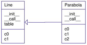
$Fig.\ 9.1\ \ {\rm UML}$  diagram for the class hierarchy with superclass Line and subclass Parabola.
