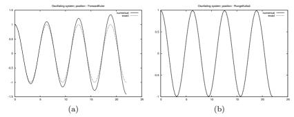
**Fig. 9.8** Solution of an oscillating system (u'' + u = 0 formulated as system of two ODEs) by (a) the Forward Euler method with  $\Delta t = 2\pi/200$ ; and (b) the 4-th order Runge-Kutta method with  $\Delta t = 2\pi/20$ .
