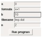
Fig. 9.14 Screen dump of a graphical user interface to read input data into a program (class GUI in the ReadInput hierarchy).
