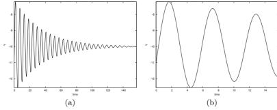
**Fig. C.3** Plot of the position of an oscillating box where the end point of the spring (w(t)) is given a sudden movement at t=0. Other parameters are m=k=1,  $\beta=0.1$ , g=0,  $S_0=0$ . (a) 1000 time steps; (b) 100 steps for magnifying the first oscillation cycles.
