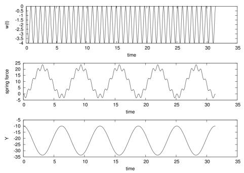
**Fig. C.4** Plot of the plate position w(t), the spring force (proportional to S(t)), and the position Y(t) for a test problem where  $w(t) = 2(\cos(8t) - 1)$ ,  $\beta = g = 0$ , m = k = 1,  $S_0 = 0$ ,  $\Delta t = 0.5236$ , and N = 600.
