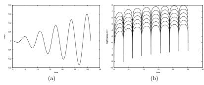
Fig. C.5 Error plots for a test problem involving an oscillating system: (a) the error as a function of time; (b) the logarithm of the absolute value of the error as a function of time, where  $\Delta t$  is reduced by one half from one curve to the next one below.
