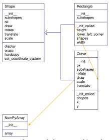
Fig. 9.12 UML diagram of parts of the shapes hierarchy. Classes Rectangle and Curve are subclasses of Shape. The darkest arrow with the biggest arrowhead indicates inheritance and is-a relationship: Rectangle and Curve are both also Shape. The lighter arrow indicates has-a relationship: Rectangle has a Curve, and a Curve has a NumPyArray.
